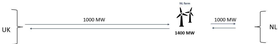
Figure 6-12: Schematic representation of a connection scenario including a Dutch wind farm with a cross-border connection.
