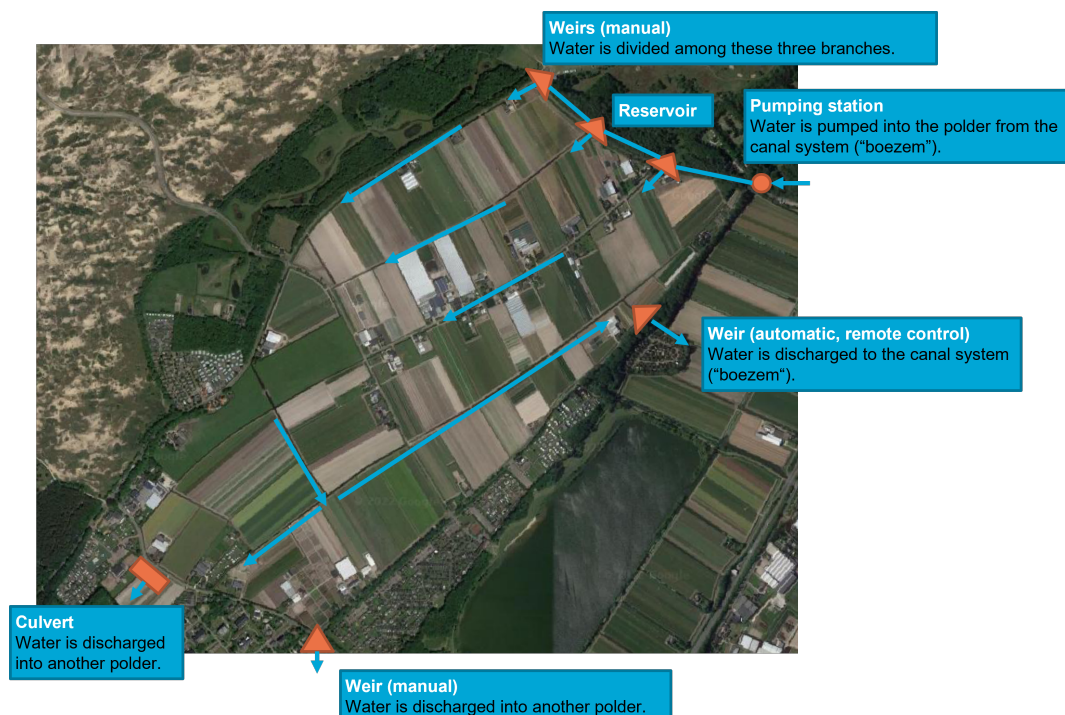
Figure 4.11: Location of the most important weirs and pumping stations in Polder Het Langeveld. Water flow directions are also indicated.
