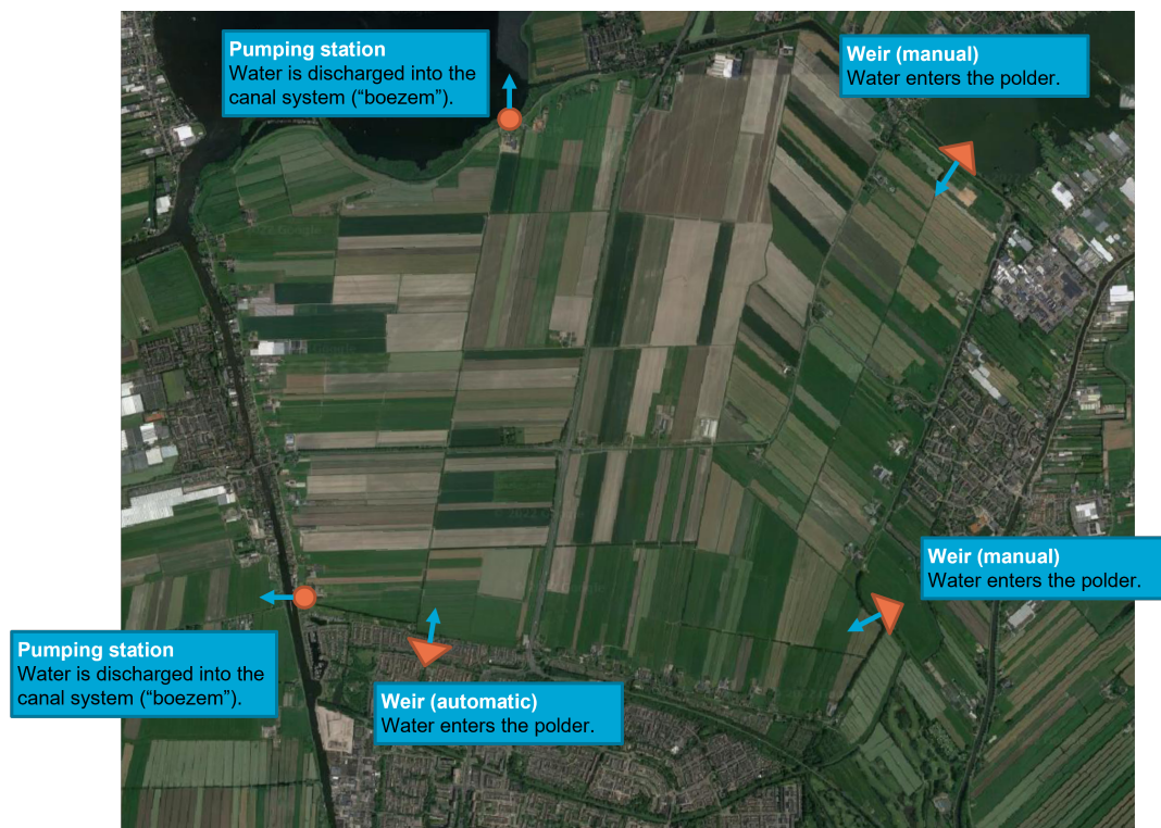
Figure 4.15: Location of the most important weirs and pumping stations in Polder Vierambacht. Water flow directions are also indicated.
