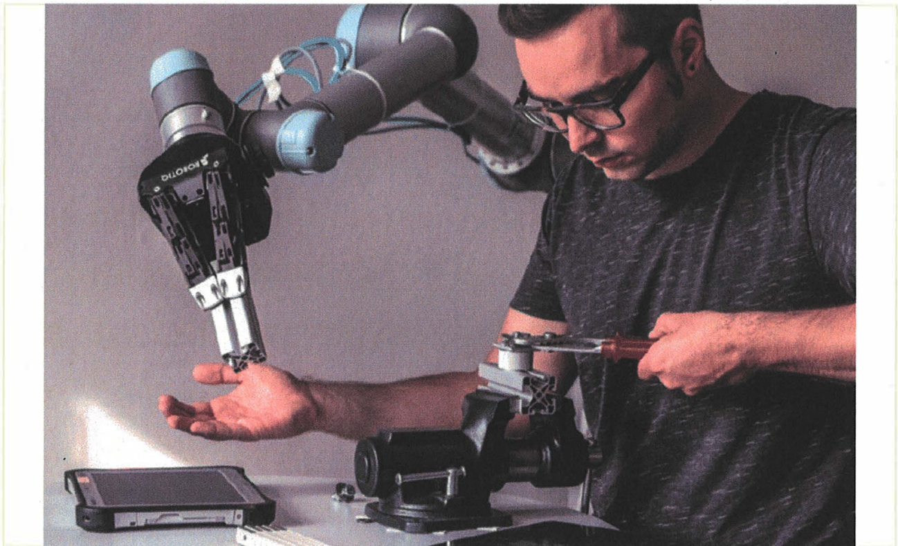
image / figure 1 A collaborative robot assisting an operator in an assembly task. (Gervasi et al., 2020)
