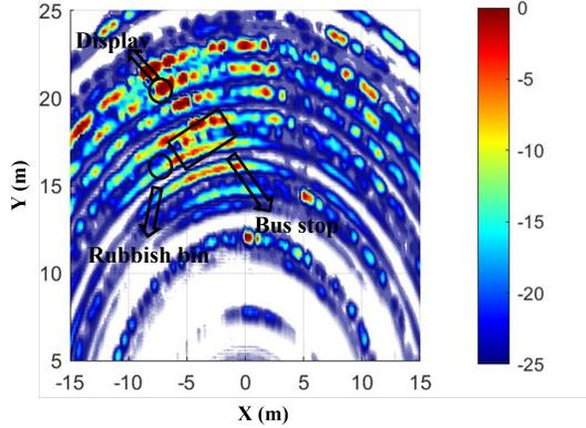
Fig. 3: The radar imaging results using all 86 elements.
