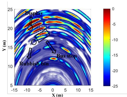
Fig. 4: The radar imaging results using only 8 elements.
