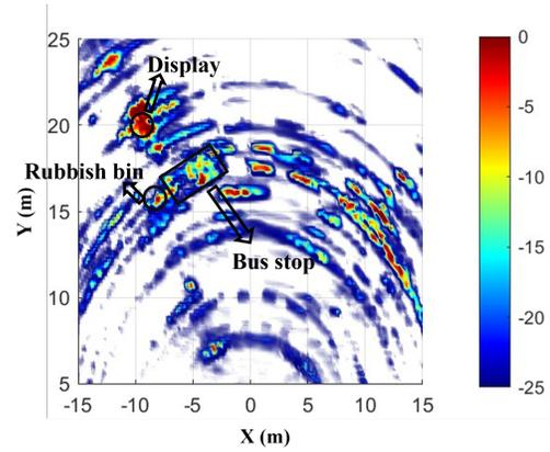
Fig. 5: The imaging results using 8 elements with the proposed 3DRUDAT algorithm.
