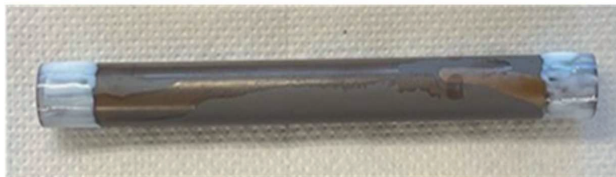
Figure S3.1. SiC coated membranes after ageing in NaClO for 200hrs.
