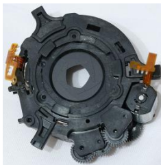
Fig. 1 Aperture mechanism of Canon 50mm f/1.8 II lens
