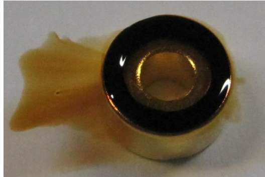
Fig. 16 Ferrofluid on glass plate above permanent magnet
