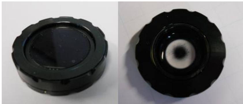
Fig. 18 Aperture demonstrator shows a black spot in the center
