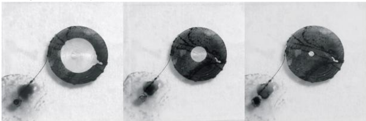
Fig. 10 Fribourg University, Dynamic microfluidic spiral iris (Müller, 2010)
