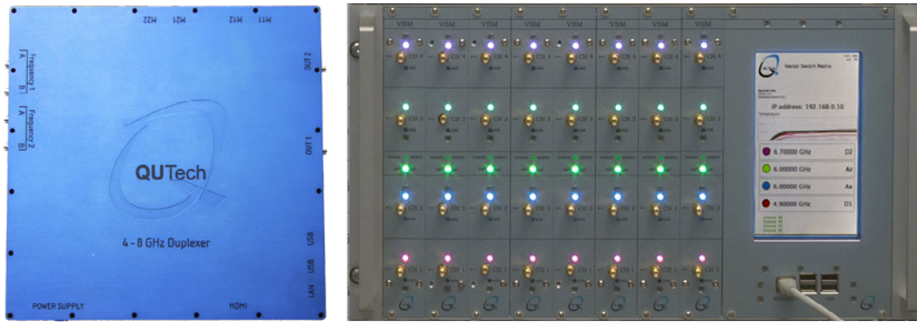
Figure 7.1: 2 frequency input, 2 qubit output VSM prototype and 4 frequency input, 32 qubit output final device aimed to save hardware for the 17 and 49-qubit surface code chips. Two prototypes have been produced so far and are being integrated into experiments.
