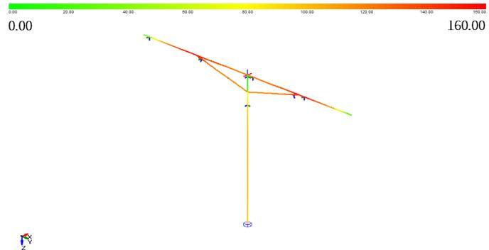
Figure 16.5: Von Mises Stress in MPa for Load Case 1
