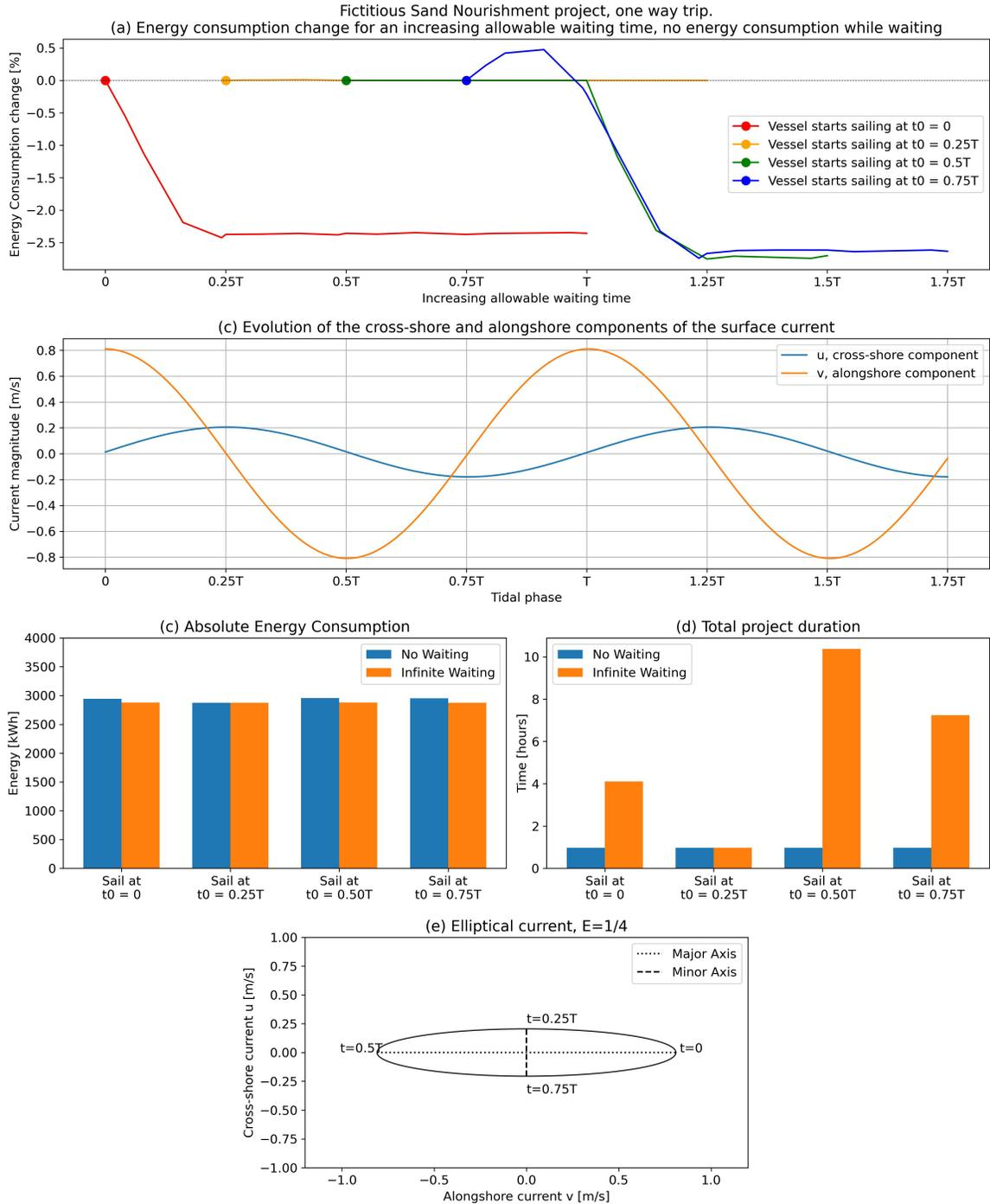
Figure D.1: Results for sailing a one way trip. Relative energy consumption change compared to no allowable waiting time for four different starting times (a), cross-shore and alongshore components at  $x = -20\text{km}$  (b), absolute energy consumption change (c) and total project duration (d). Ellipticity  $E = 1/4$  (e).
