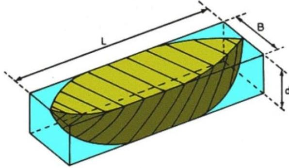
Figure 3.2: Underwater volume of hull in yellow, rectangular underwater block volume in blue (Maritmeculture, 2020)
