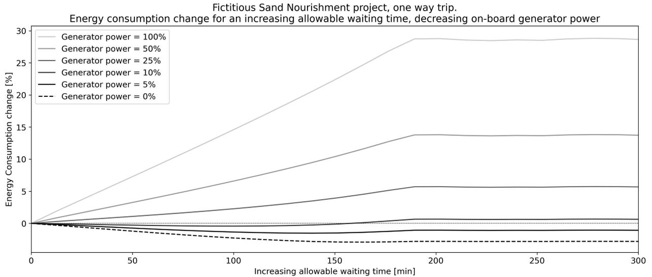
Figure 4.16: Results for a one way trip from deep water to the coast. Relative energy consumption reduction for a decreasing generator power.
