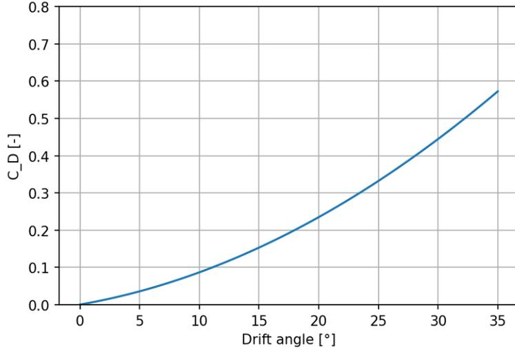
Figure 3.7: Drag coefficient for increasing drift angle, based on research from Lübke (2016)
