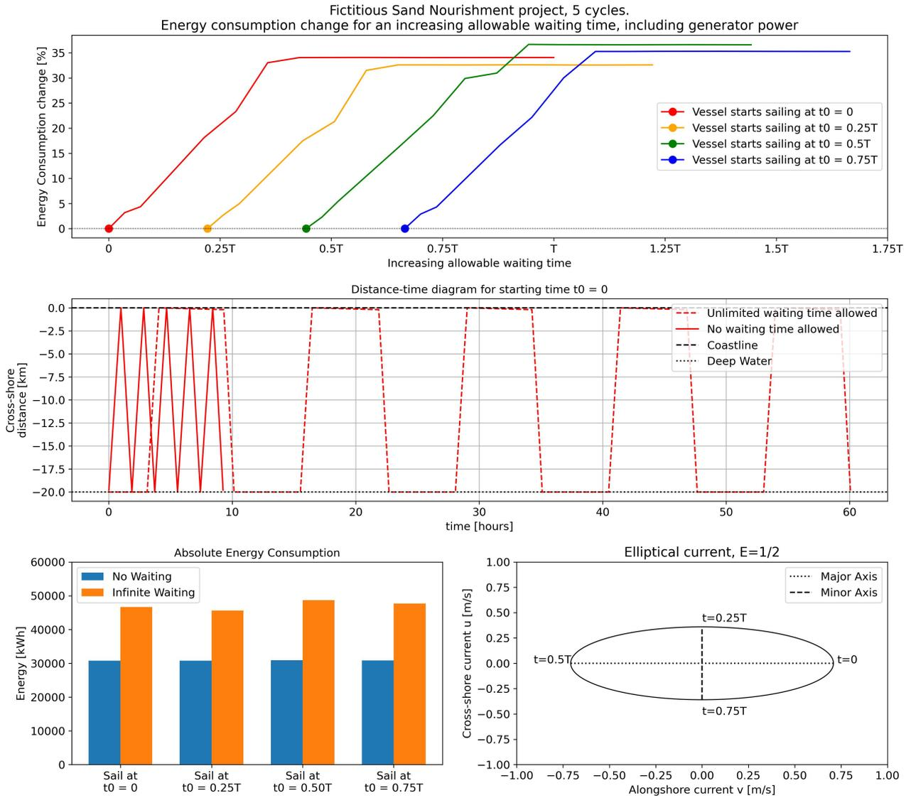
Figure 4.15: Results for sailing 5 cycles, including generator power ( $P_{generator} = 327.1$  kW). Relative energy consumption change compared to no allowable waiting time for four different starting times (top), time-distance diagram for starting time  $t_0 = 0$  (middle), absolute energy consumption change (bottom left) and ellipticity  $E = 1/2$  (bottom right).
