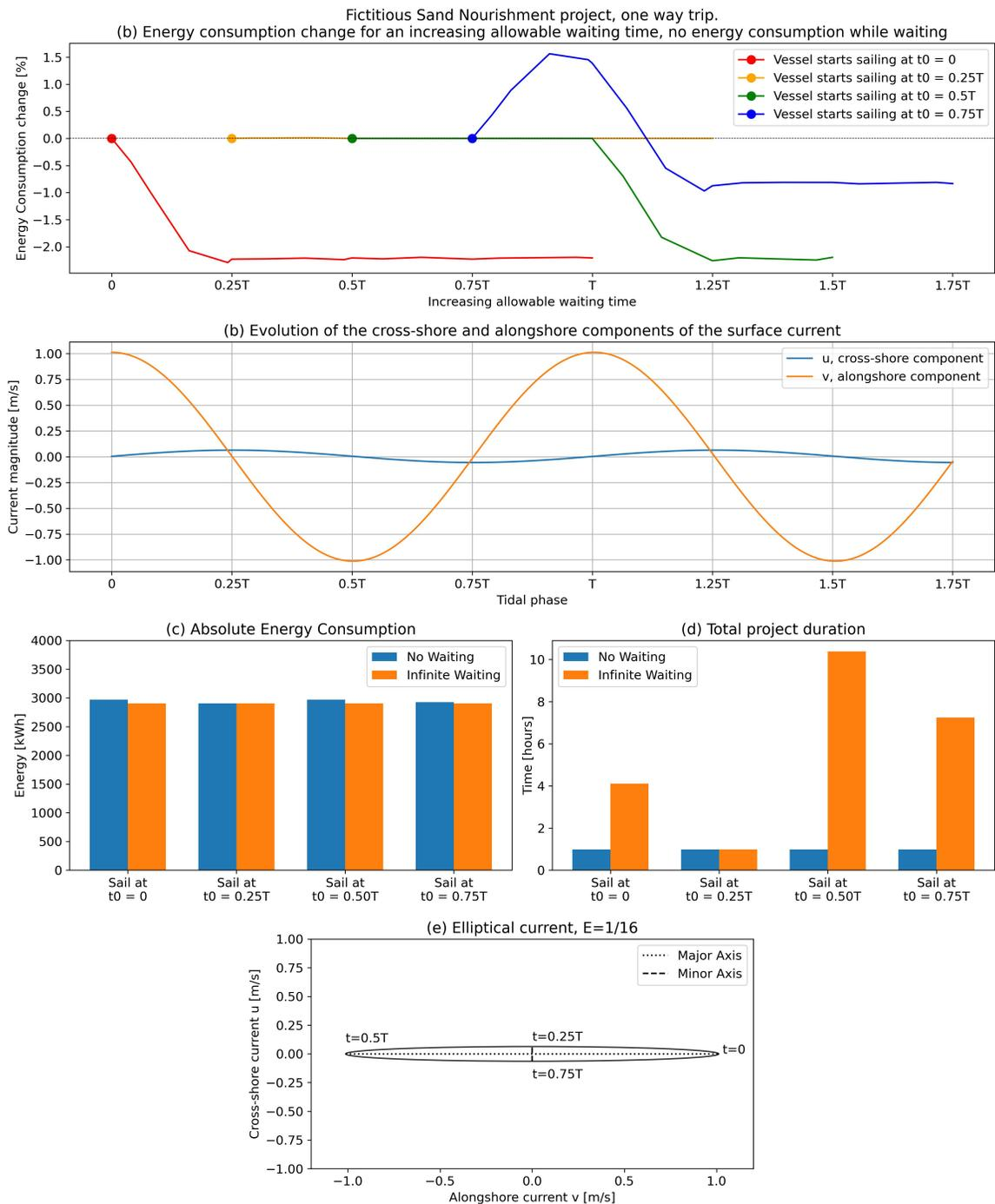
Figure D.3: Results for sailing a one way trip. Relative energy consumption change compared to no allowable waiting time for four different starting times (a), cross-shore and alongshore components at  $x = -20\text{km}$  (b), absolute energy consumption change (c) and total project duration (d). Ellipticity  $E = 1/16$  (e).
