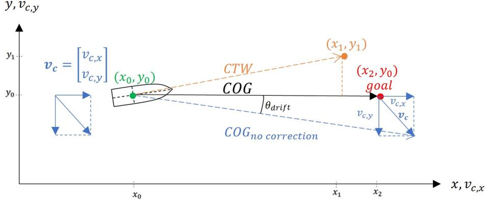
Figure 3.12: Scenario 3: sailing in x-direction, current has a perpendicular and parallel component
