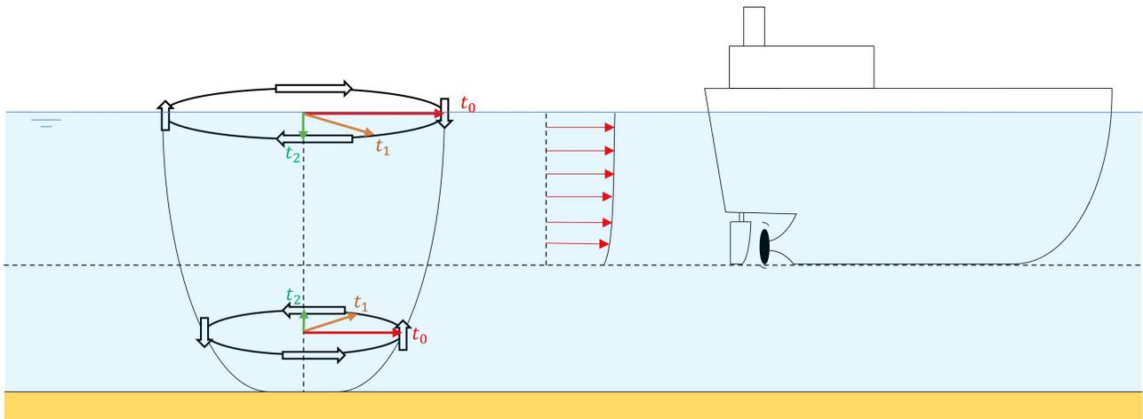
Schematization of a dredging vessel sailing through the vertical velocity structure (left), with counter-rotating elliptical currents at the surface and bed, and the part affecting the vessel at  $t_0$  (middle).
