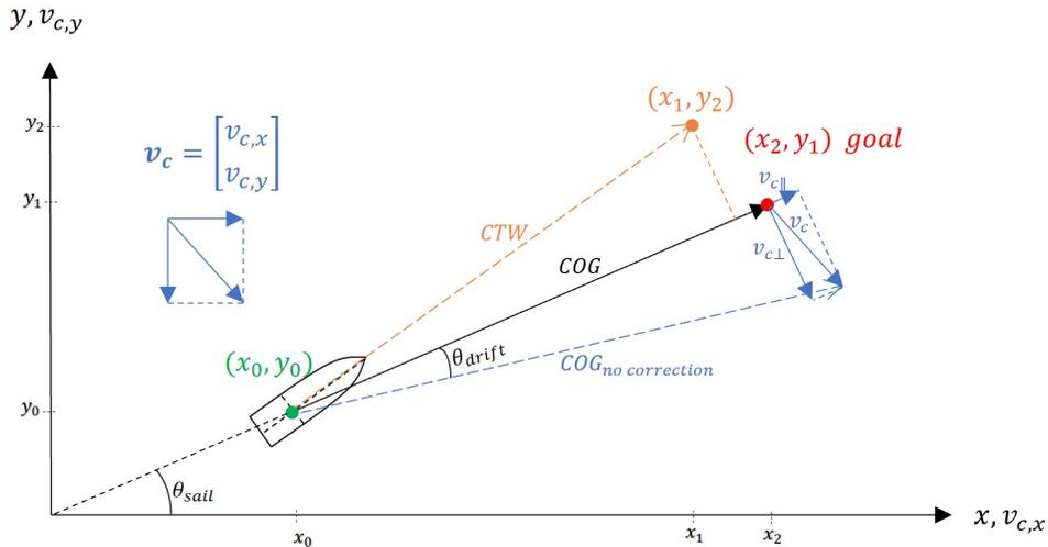
Figure 3.13: Scenario 4: Both the sailing direction and the current have a x- and y-component
