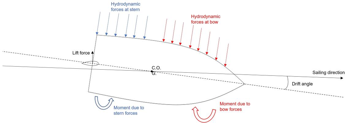
Figure 3.6: Top view of a sailing vessel, including bow and stern moments caused by hydrodynamic forces along the vessel
