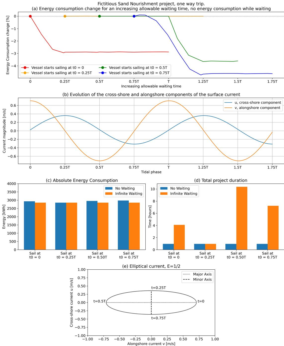
Figure 4.12: Results for sailing a one way trip. Relative energy consumption change compared to no allowable waiting time for four different starting times (a), cross-shore and alongshore components at  $x = -20\text{km}$  (b), absolute energy consumption change (c) and total project duration (d). Ellipticity  $E = 1/2$  (e).
