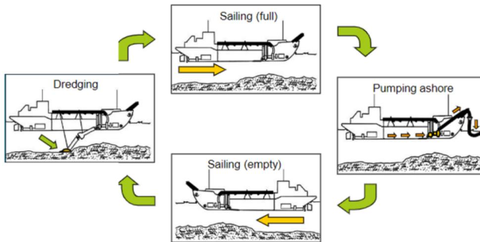
Figure 4.7: Four stages of a typical dredging cycle; dredging, sailing full, dumping (pumping ashore) and sailing empty. (Lamers, 2022)
