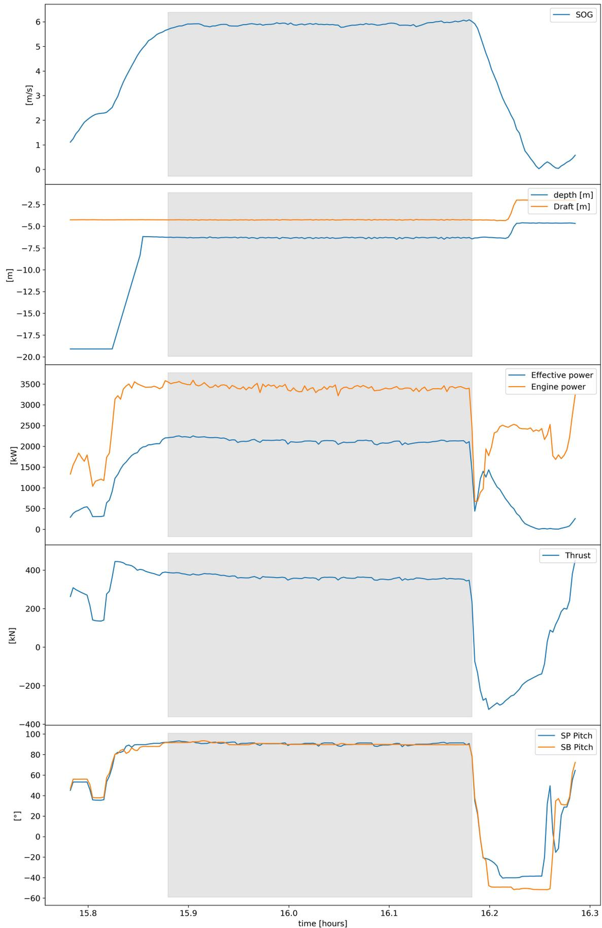
Figure 4.5: Validation criteria check for Vessellog data. The dredging vessel sails from the deep dredged channel to shallows next to the channel.
