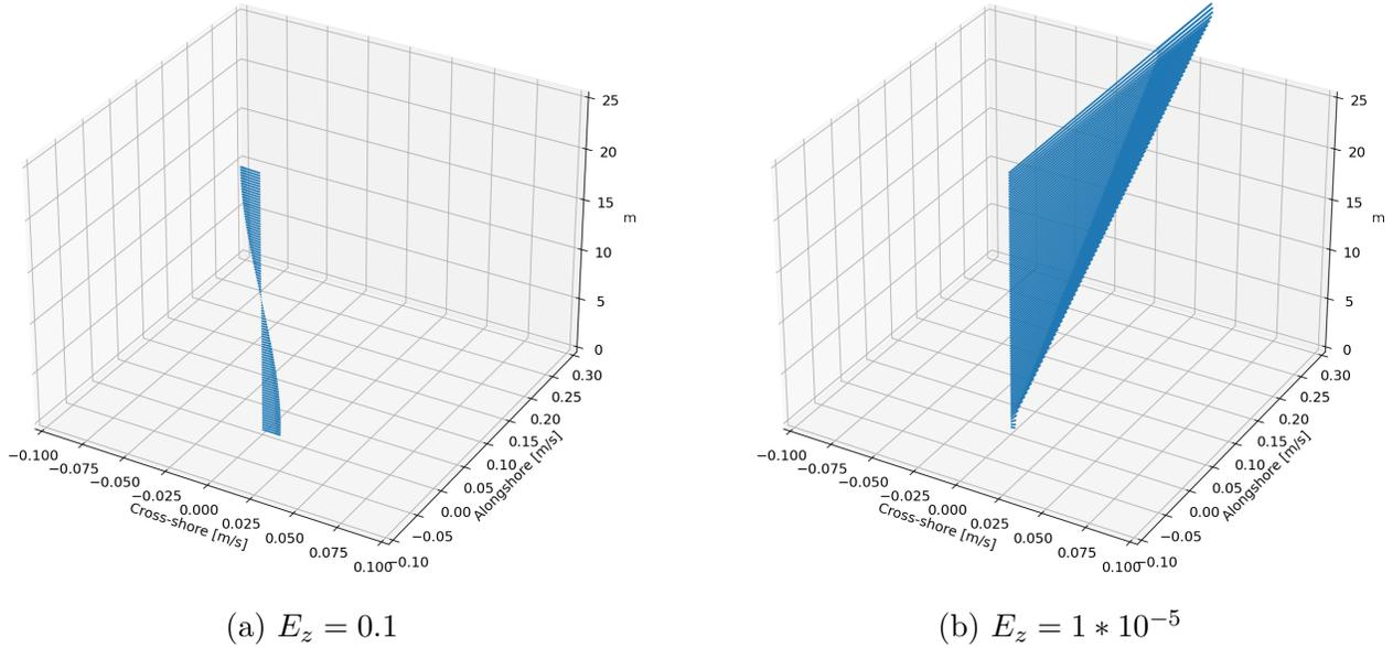
Figure 2.4: Vertical structure Heaps for low and high mixing energy
