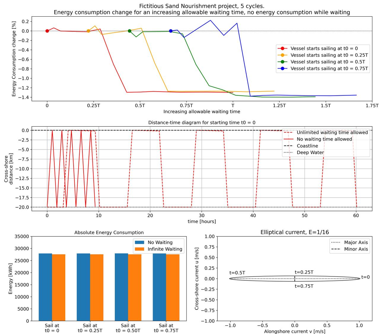
Figure D.6: Results for sailing 5 cycles. Relative energy consumption change compared to no allowable waiting time for four different starting times (top), cross-shore and alongshore components at  $x = -20\text{km}$  (middle), absolute energy consumption change (bottom left) and ellipticity  $E = 1/16$  (bottom right).
