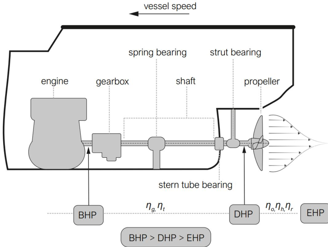
Figure 3.1: Schematization of relation between brake horse power, delivered horse power and effective horse power. (Koningsveld et al., 2021)
