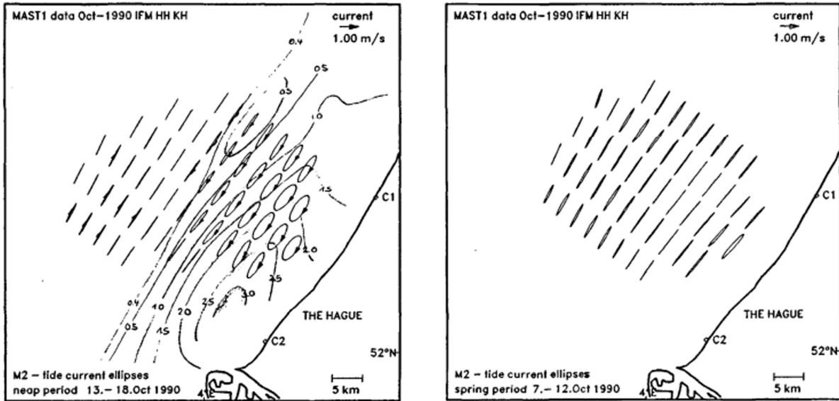
Figure 4.11: Surface tidal current ellipses calculated from CODAR data from records. A neap tide or stratified scenario (left) and a spring tide or well mixed scenario (right). (Visser et al., 1994)
