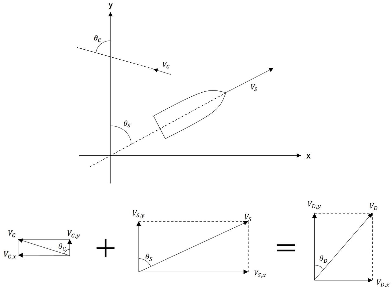
Figure 3.8: Top view of STW magnitude and angle and current magnitude and angle (upper), vector addition (lower). Where  $V_S = \text{STW [m/s]}$ ,  $\theta_S = \text{STW angle [}^\circ\text{]}$ ,  $V_C = \text{current magnitude [m/s]}$ ,  $\theta_C = \text{current angle [}^\circ\text{]}$ ,  $V_D = \text{Deviation sailing speed, i.e. SOG [m/s]}$ ,  $\theta_D = \text{Deviation angle, i.e. SOG angle [}^\circ\text{]}$ .
