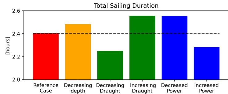
Figure 4.2: Test cases 1-4: respectively the reference case, varying the water depth  $D$ , varying the draught  $T$  and varying the engine power  $P_b$
