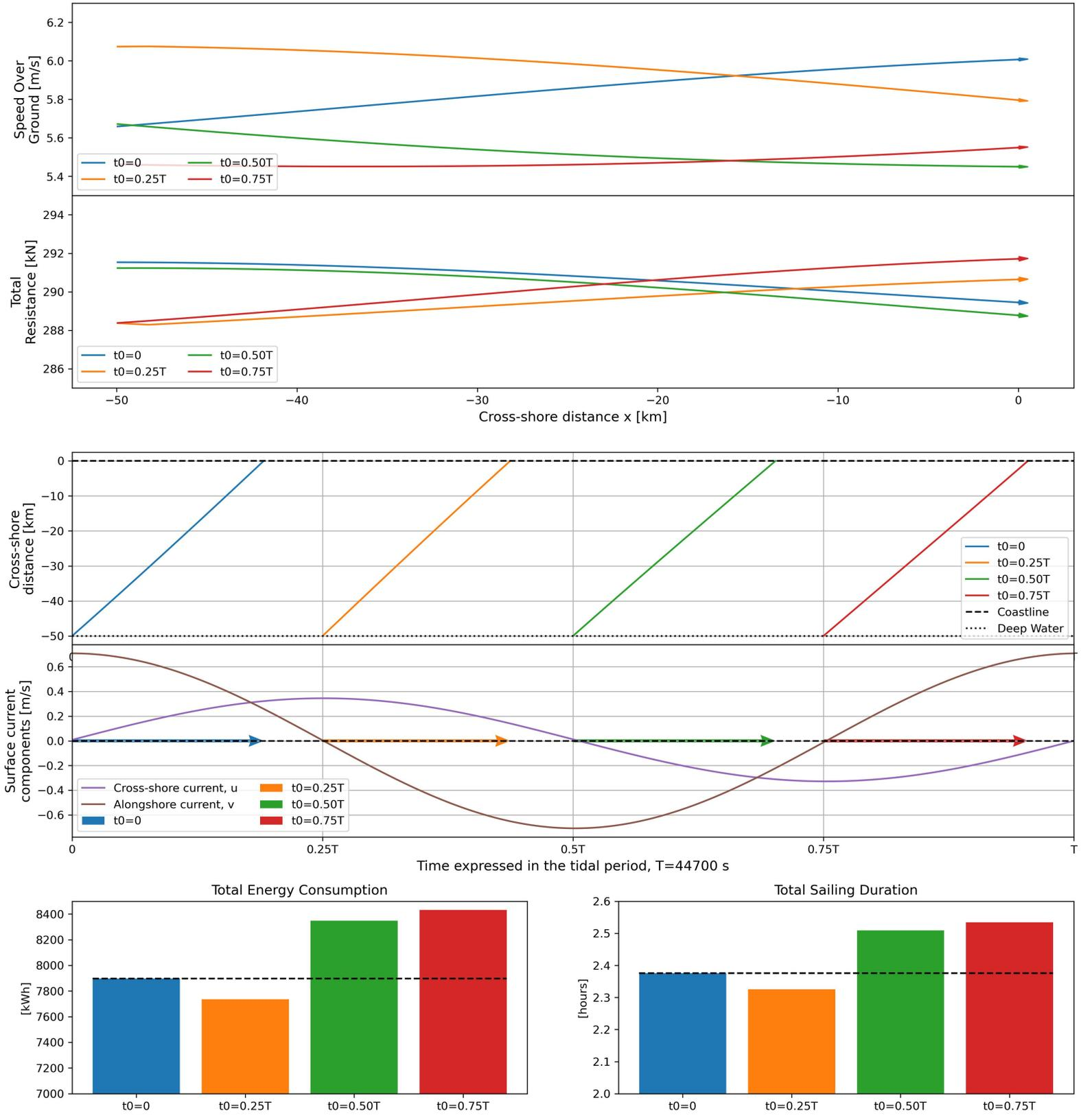
Figure 4.4: Test case 6: Prandle and Heaps flow field, varying the starting time
