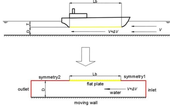
Figure 3.3: Simplification of a vessel in shallow water illustrating the sailing speed  $V$  and increased water velocity  $V_B (=V + \Delta V)$  (Zeng et al., 2019)
