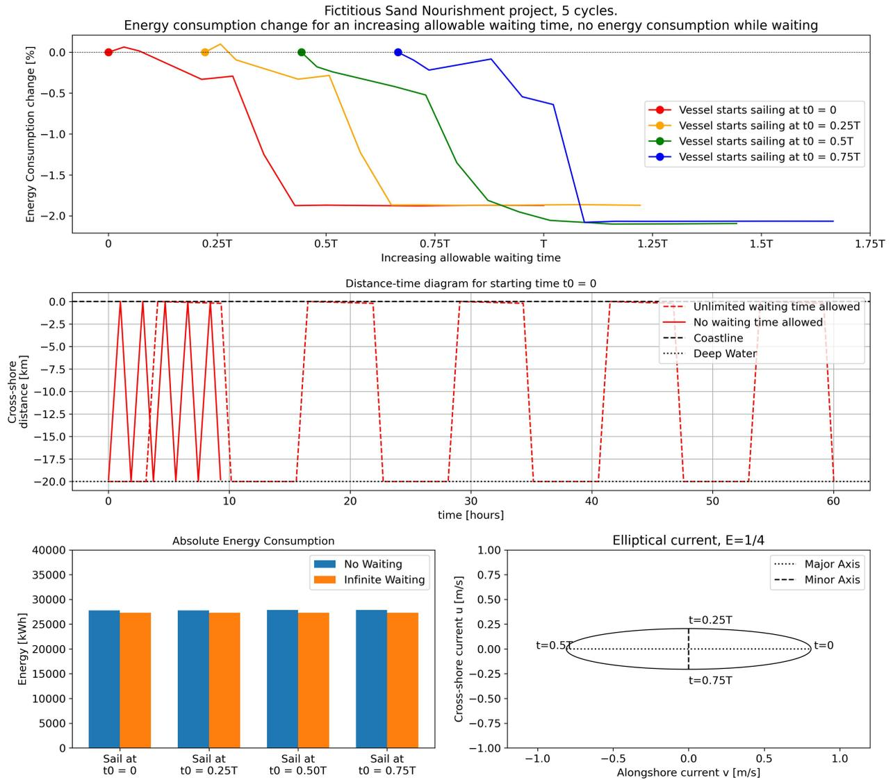
Figure D.4: Results for sailing 5 cycles. Relative energy consumption change compared to no allowable waiting time for four different starting times (top), cross-shore and alongshore components at  $x = -20\text{km}$  (middle), absolute energy consumption change (bottom left) and ellipticity  $E = 1/4$  (bottom right).
