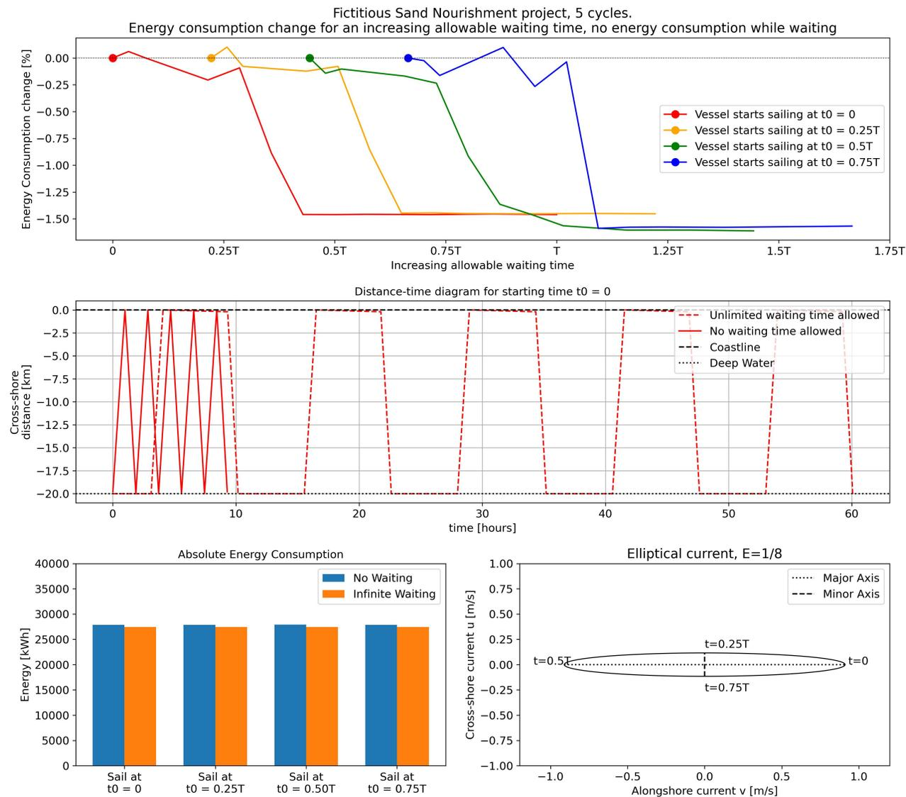
Figure D.5: Results for sailing 5 cycles. Relative energy consumption change compared to no allowable waiting time for four different starting times (top), cross-shore and alongshore components at  $x = -20\text{km}$  (middle), absolute energy consumption change (bottom left) and ellipticity  $E = 1/8$  (bottom right).
