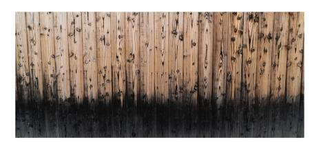
CHARRING WOOD FOR WEATHERPROOFING SOURCE: NAKOMOTOFORESTRY.COM
