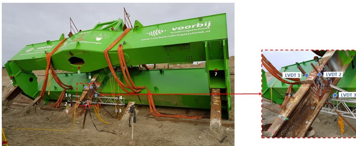
Figure 3.5: Schematic overview and pictures of testing frame and relevant components (personally taken photograph: Putteman, J.)
