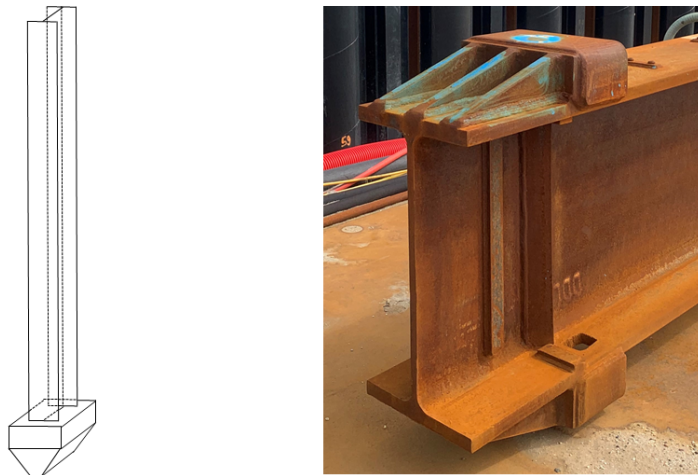
Figure 2.2: Schematisation of MV pile (left) and picture of pile tip (right).
