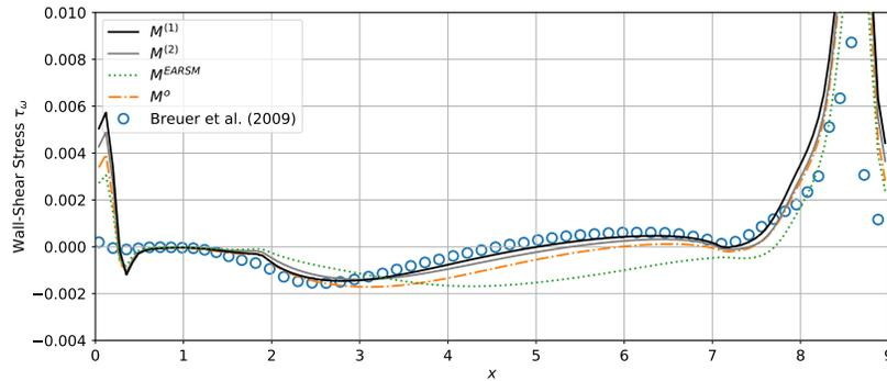
**Fig. 5 Prediction of the wall-shear stress for  $Re_H = 10595$  using correction models  $M^{(1)}$  and  $M^{(2)}$ ,  $k-\omega$  LEVM  $M^o$  and EARSM  $M^{EARSM}$  from literature [24]. Validation data from [19].**
