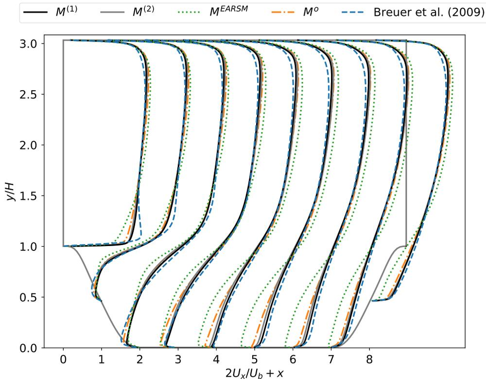
**Fig. 4** Predictions of the stream-wise velocity for  $Re_H = 10595$  using correction models  $M^{(1)}$  and  $M^{(2)}$ ,  $k - \omega$  LEVM  $M^o$  and EARSM  $M^{EARSM}$  from literature [24]. Validation data from [19].
