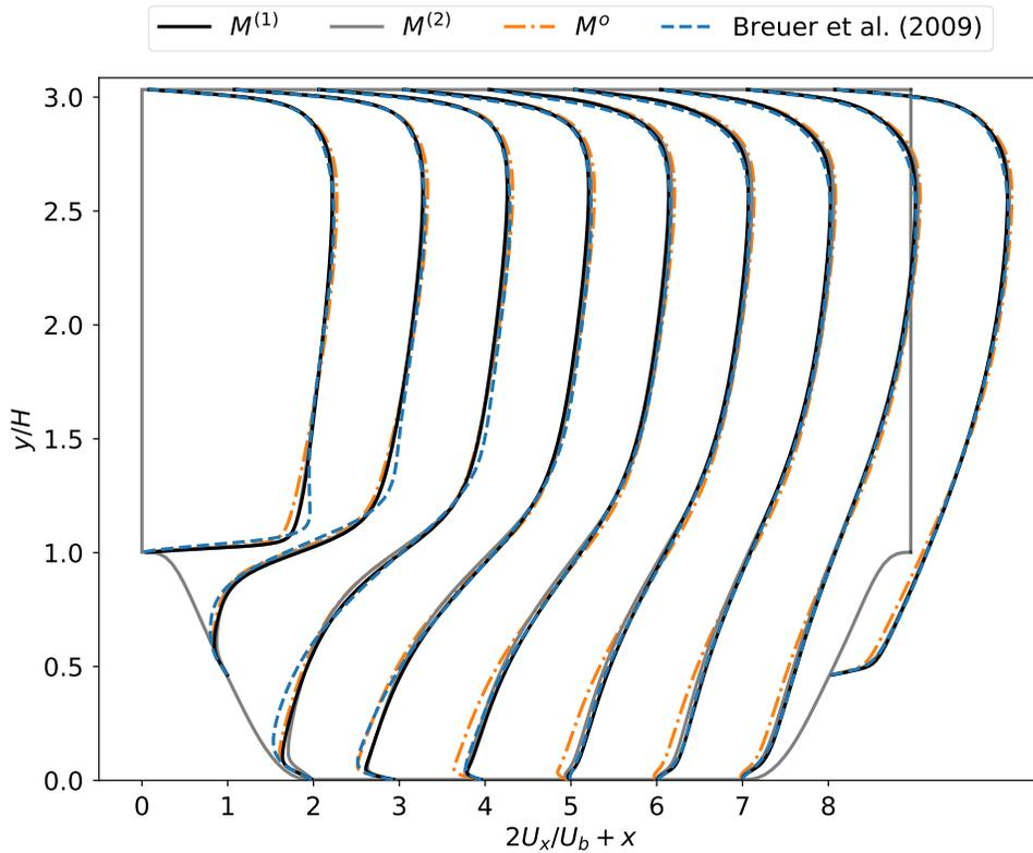
**Fig. 6 Predictions of the stream-wise velocity for  $Re_H = 2800$  using correction models  $M^{(1)}$  and  $M^{(2)}$  and  $k-\omega$  LEVM  $M^o$ . Validation data from [19].**
