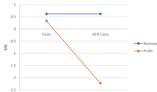
Figure 4.6: Effect of increasing system costs for a 200MWh/110MW flow battery simulated for one week.
