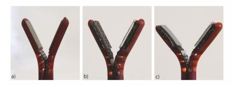
Figure 9.4: The three fabricated grippers. The reference gripper (a) was equipped with a grooved stainless-steel plate. In unpatterned pads (b), the elastomeric pads appear transparent, whereas in patterned pads (c), a white haze can be seen at the pad surface. In soft pads, either patterned or unpatterned, the CFF was embedded in the elastomeric pad.
