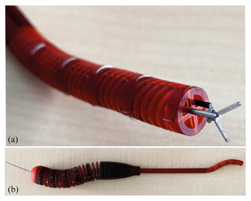
Figure 5.8: Pictures of the HelicoFlex prototype. (a) Close-up of the compliant shaft of the HelicoFlex with a flexible biopsy forceps in one lumen and a flexible fiber optics endoscope in the second; (b) bendable metal rod inserted into one of the lumens to create a certain shape in the compliant shaft and keep it in position.
