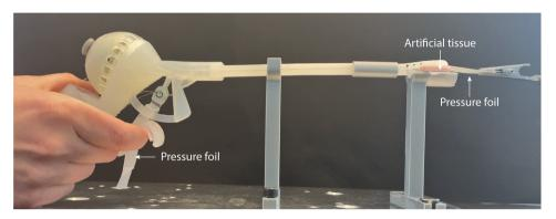
Figure 7.11: Set-up of the grasping force measurement.
