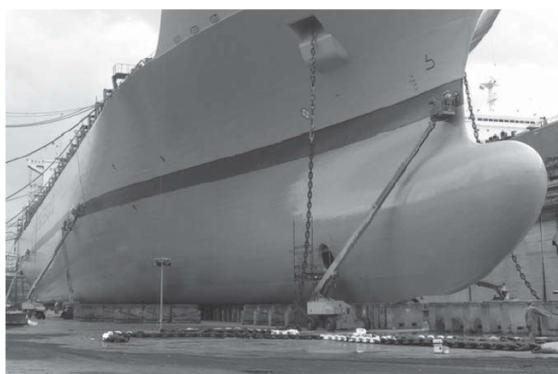
Figure 1.1: picture of a container vessel equipped with a bulbous bow. Ridley (2014)
