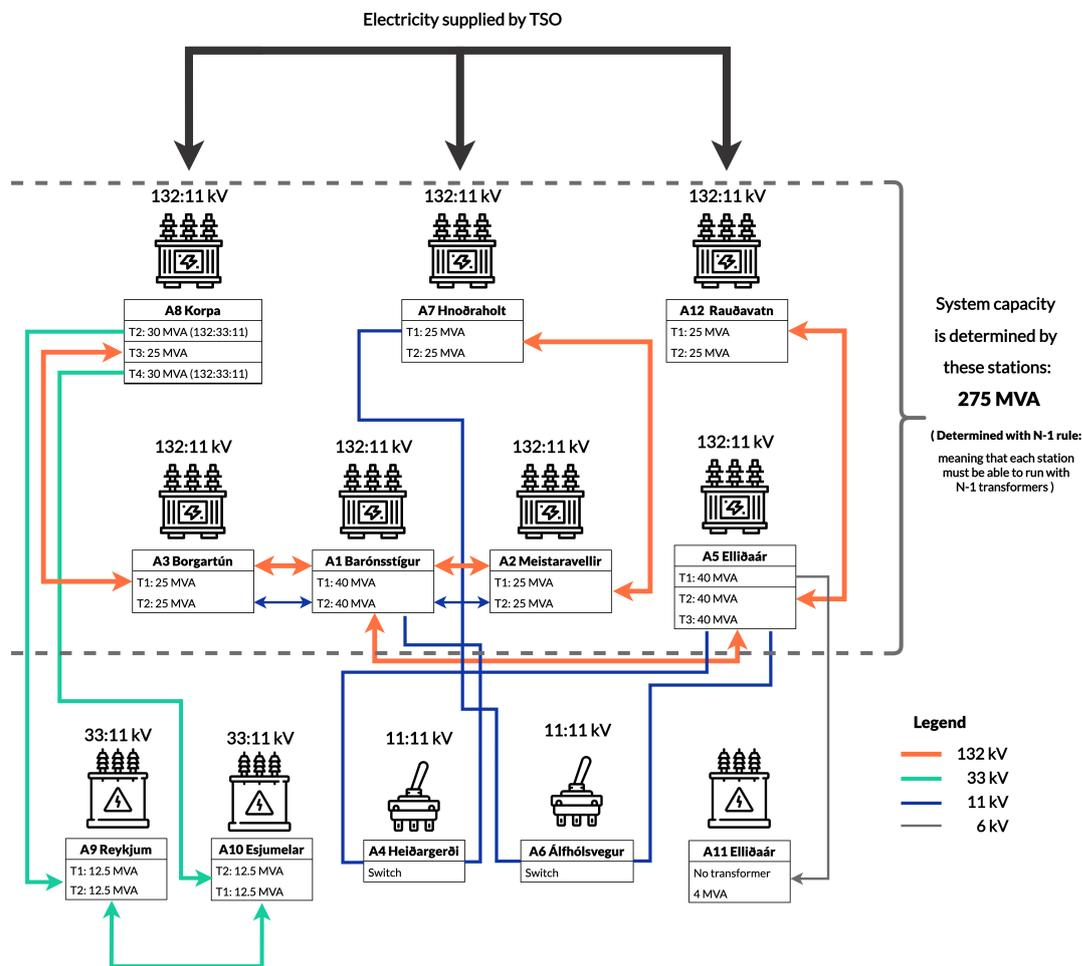
Figure 5.6: Overview of the connections between the high voltage substations and how the global distribution grid capacity limit is determined. Based on a system schematic provided by the DSO. Icons from www.flaticon.com
