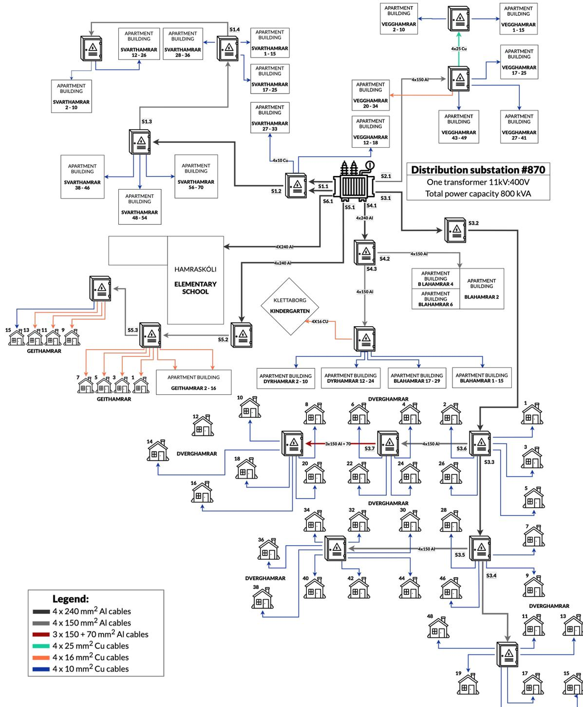
Figure 5.8: Visualised schematic of the local grid behind distribution substation 670. Different colors of cables mean different materials and thus capacity. These cable materials are explained in the legend in the figure. Icons from www.flaticon.com
