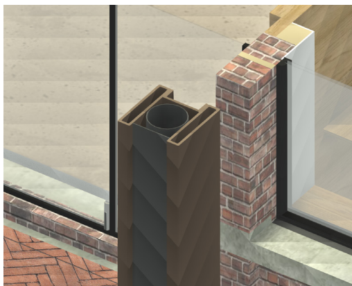
VENTILATION DUCT INTEGRATED IN COLUMN
