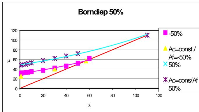
**Influence of the channel area, for different disturbances, on the system time-scale**
