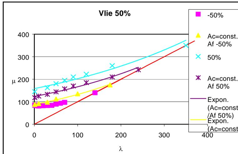
**Influence of the channel area, for different disturbances, on the system time-scale**
