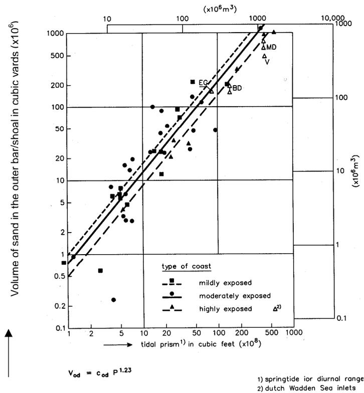
**Figure 3-5. Sand volume outer deltas in USA in relation to the mean tidal volume of the inlet, according to Walton and Adams**
