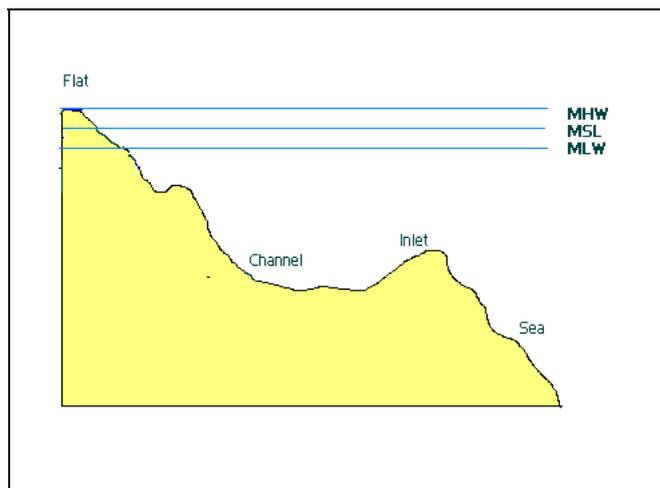
**Figure 2-6. Cross-section of a tidal inlet system**
