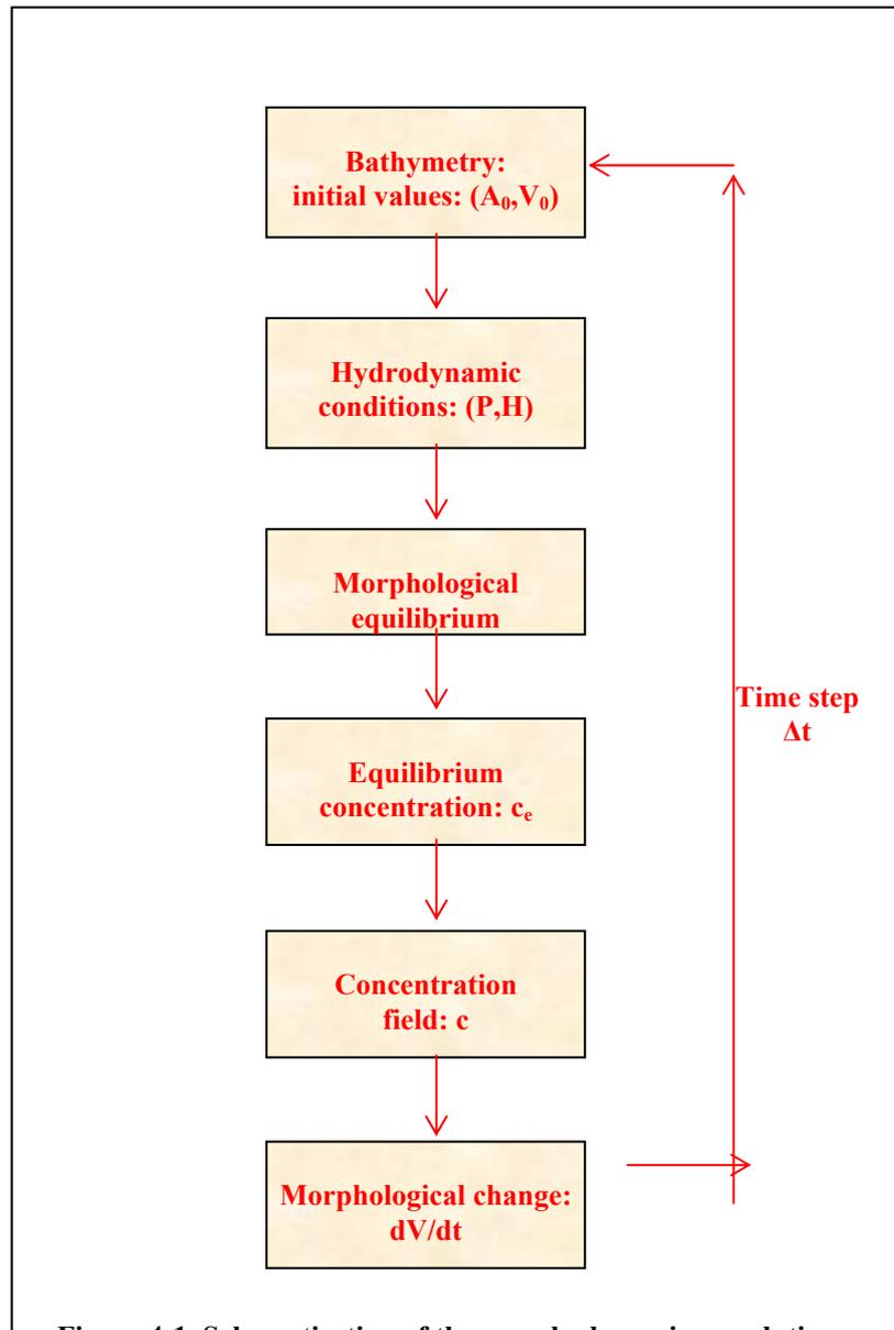
Figure 4-1. Schematisation of the morphodynamic evolution in ASMITA
