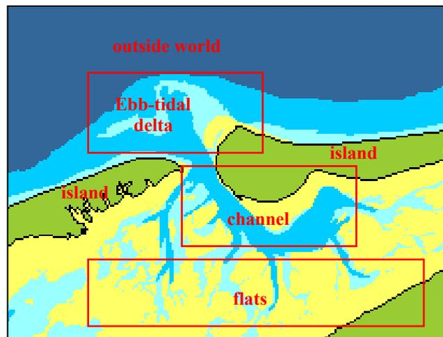
**Figure 3-1. Schematisation of tidal inlet systems**
