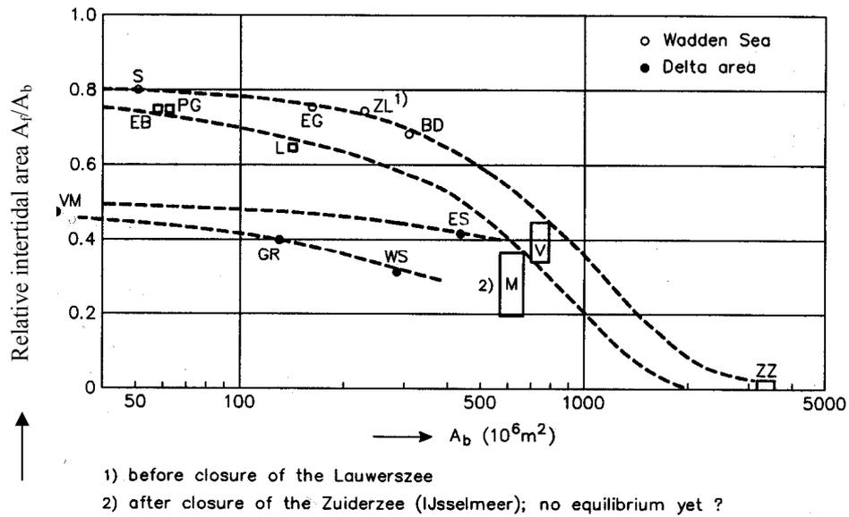
**Figure 3-6. Relative area of the intertidal zones in the Dutch Wadden Sea and delta area (*Eysink and Biegel, 1993*)**
