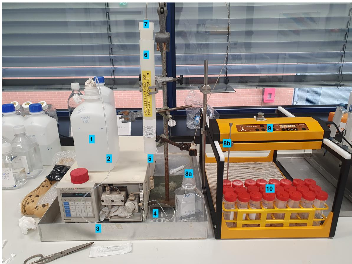
**Figure 3.2:** 1: Loading/elution solution, 2: Tubing, 3: Pump, 4: Purge tube for removing air, 5: Column inlet, 6: Column, 7: Column outlet, 8a: Tubing to waste container, 8b: Tubing to vials, 9: Fraction collector, 10: Collection vials.
