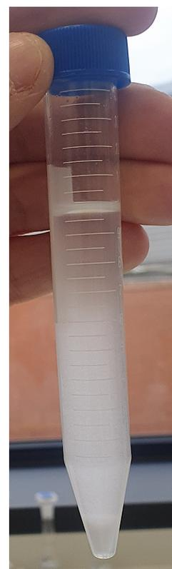
**Figure 3.1:** The DDPA/TBP solution. Not all DDPA has dissolved resulting in a cloudy solution with the undissolved DDPA powder at the bottom of the vial.
