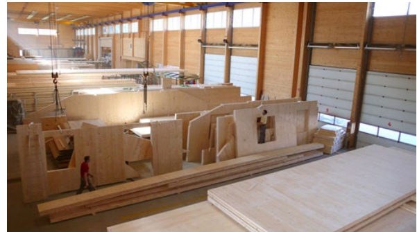
Figure 11 CLT panels with custom shape including cut outs for windows and doors [17]
