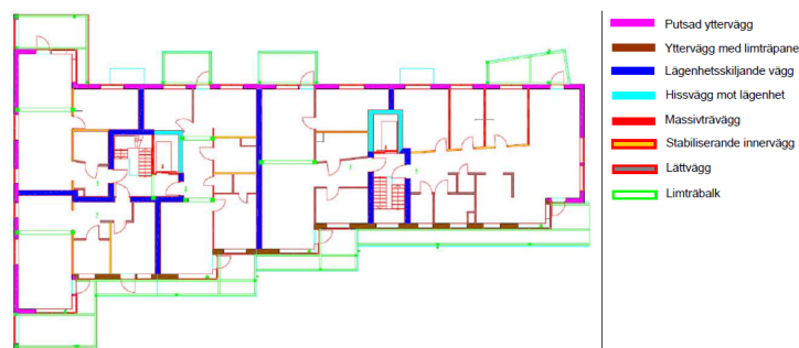
Figure 108 Walls contributing to the stability [51]
