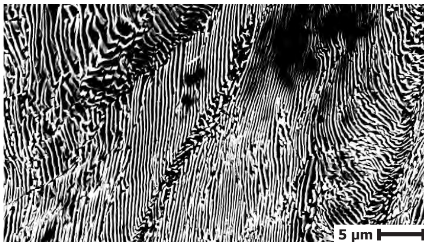
Figure 4.6. Secondary electron image of a "canal" cutting through a pearlite colony in the eutectoid steel after one pass.
