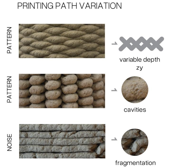
Figure 23 : Cavity formation due to printing path variation
