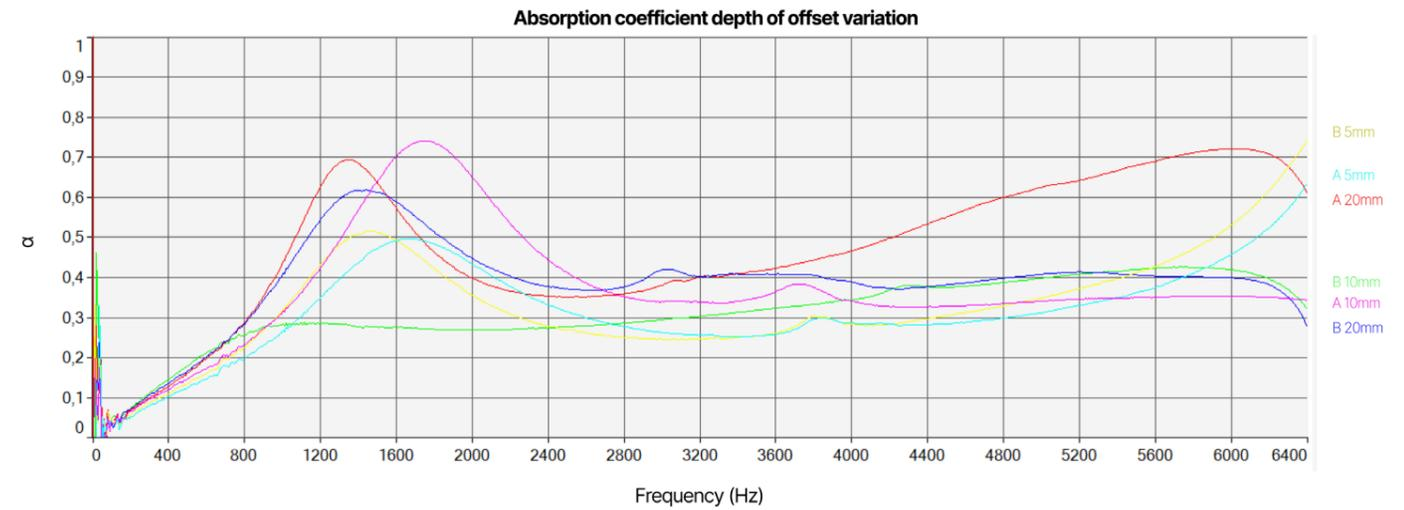
Figure 56 : Depth of offset variation high frequencies
