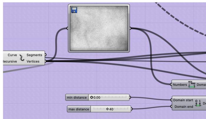
The noise was generated through image mapping. For this example a grainy image was used. The point movement distances were mapped to a maximum of 40mm. The point movement is outwards on two sides and tangent on the other two to test out the difference. To hide the seam, the prototype's polyline was spiraled using 40 points for the precision ramp.
