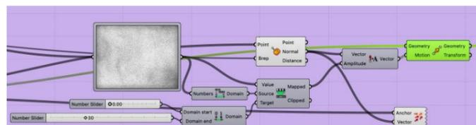
The normal vectors from the geometry were used as the directions to move the points according to the remapping from the image mapping.
