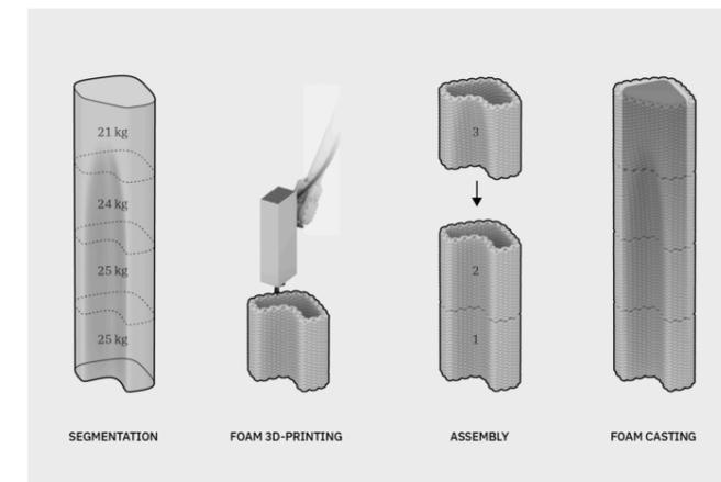
Figure 41: Design and fabrication sequence (Bedarf et al., 2023)
