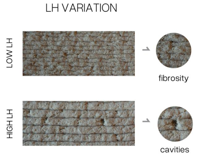
Figure 20 : Roughness in low and high layer heights
