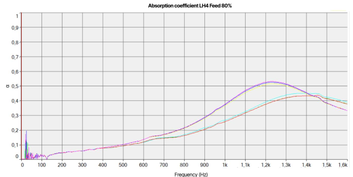
Figure xx: Comparison of absorption coefficients of the same sample (Feed 80%), replacing it in the tube for every measurement (thin loose sample)
