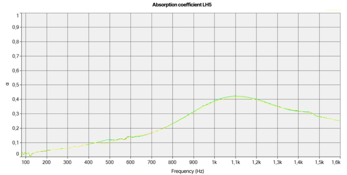
Figure xx: Comparison of absorption coefficients of the same sample (LH5), replacing it in the tube for every measurement (tightly fitting sample)
