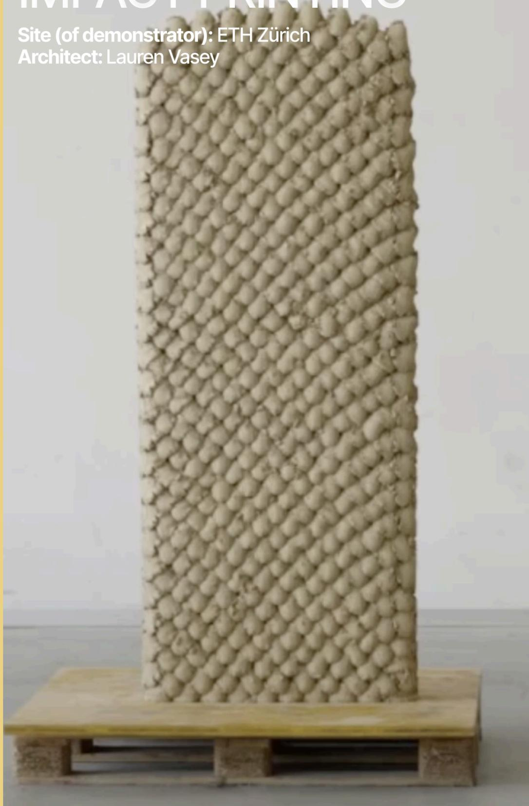
Figure 25: Vertical wall fabricated with Impact Printing (Vasey, 2024)
