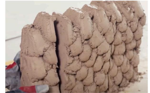
Figure 29: Seamless material connection with no dry joints (Vasey, 2024)
