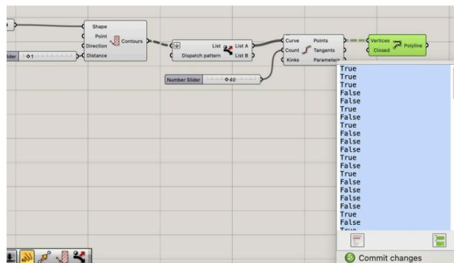
The dispatch pattern was defined so every two layer the layer height increases by 1mm
