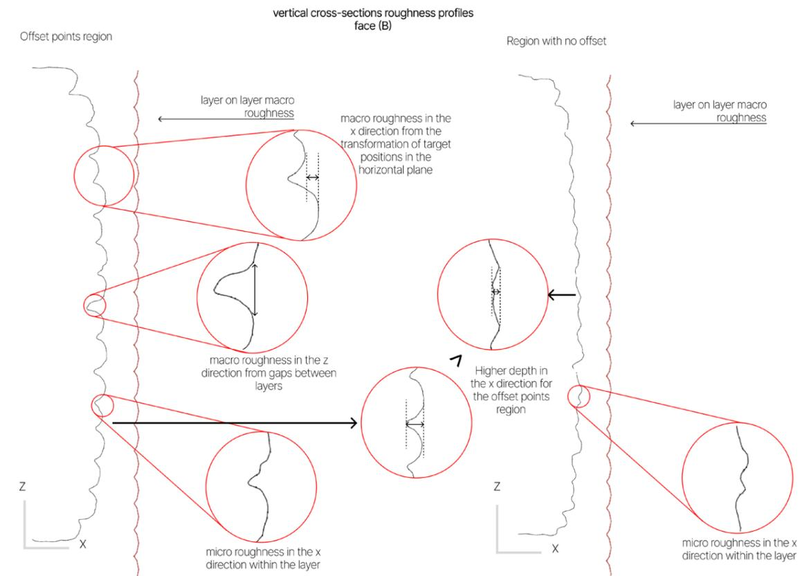
Figure 31 : Vertical cross-section roughness profile of side B
