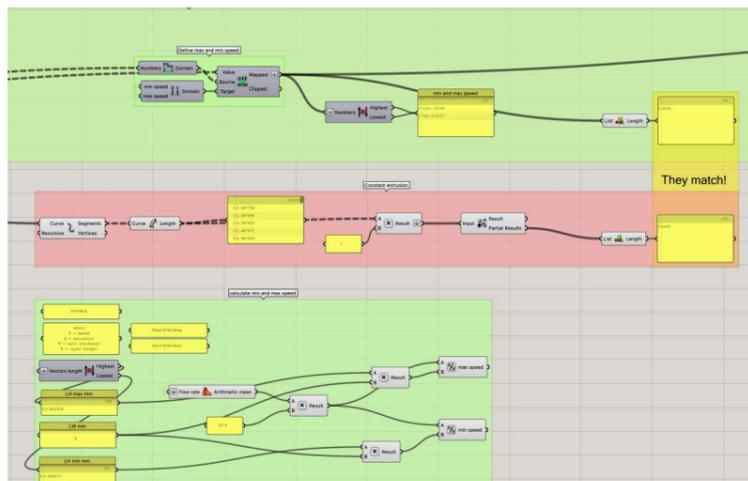
As the extrusion is defined by  $E = W * H * L / T$ , where  $Feed = LL / T$ , then we can define the the max speed as:  $F_{max} = E / W * H_{max}$ , and minimum as  $F_{min} = E / W * L_{Hmin}$ . The layer width was set as 8mm.  $F$  = speed,  $E$  = extrusion,  $W$  = wall thickness,  $H$  = layer height,  $T$  = time, and  $L$  = layer length.
