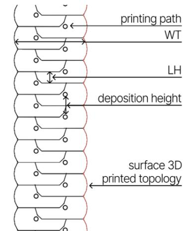
Figure 24 : Section of vertically 3D-printed parts with horizontal target position variations
