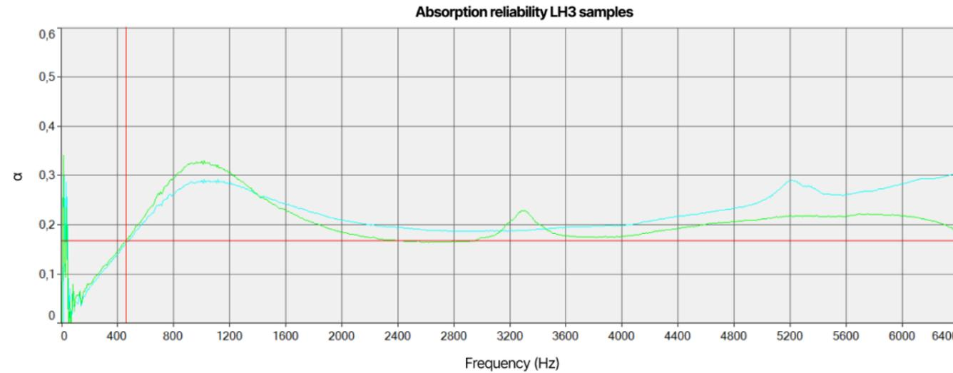
Figure xx: Comparison of absorption coefficients of two LH3 mm samples
