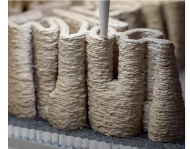
Figure 33: Prototype printing (Costalonga, 2024)
