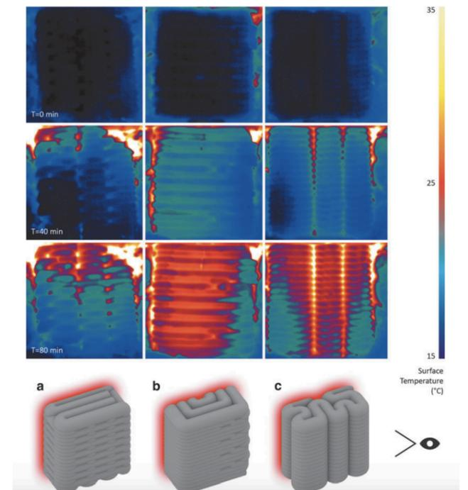
Figure 42: Thermographic comparison of infill schemes after 0, 40, and 80 min (Bedarf et al., 2023)
