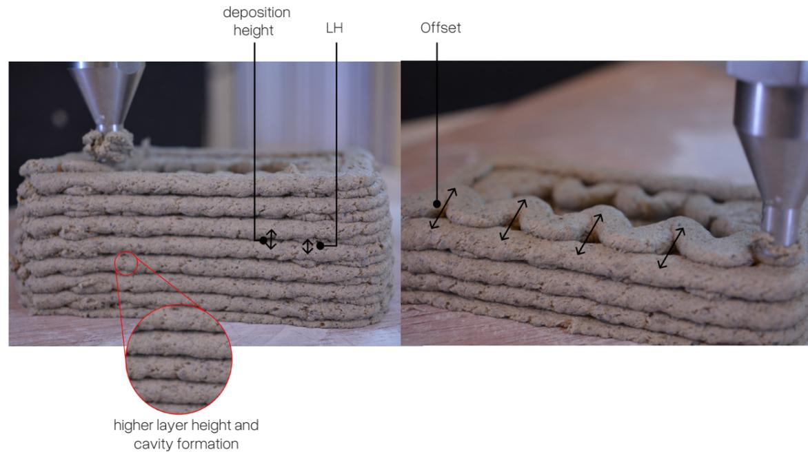
Figure 28 : Printing path manipulation approach for cavity formation
