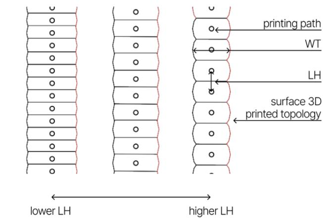
Figure 21: Section of vertically 3D-printed parts with different layer heights
