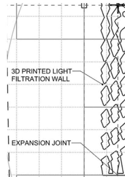
Figure 17: Wall inner geometry (Arquitectura Viva, 2024)
