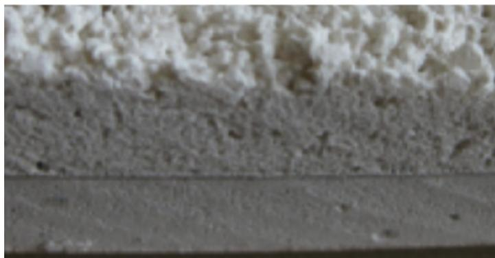
Figure 9 : Acoustical plaster on gypsum base (Binggeli, 2008)
