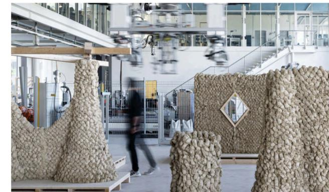
Figure 30: Impact printed structures (Chadha et al., 2024)
