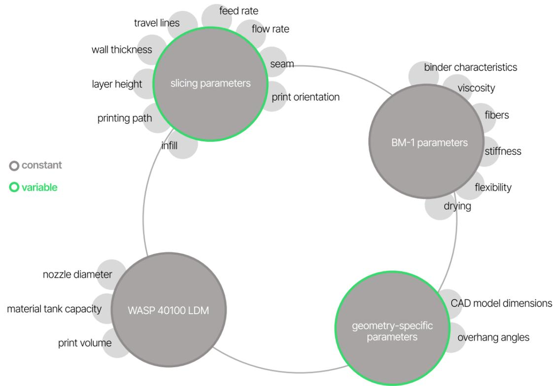
Figure 13 : Paramerts influencing the 3D printing process with BM-1, constant and variable parameters
