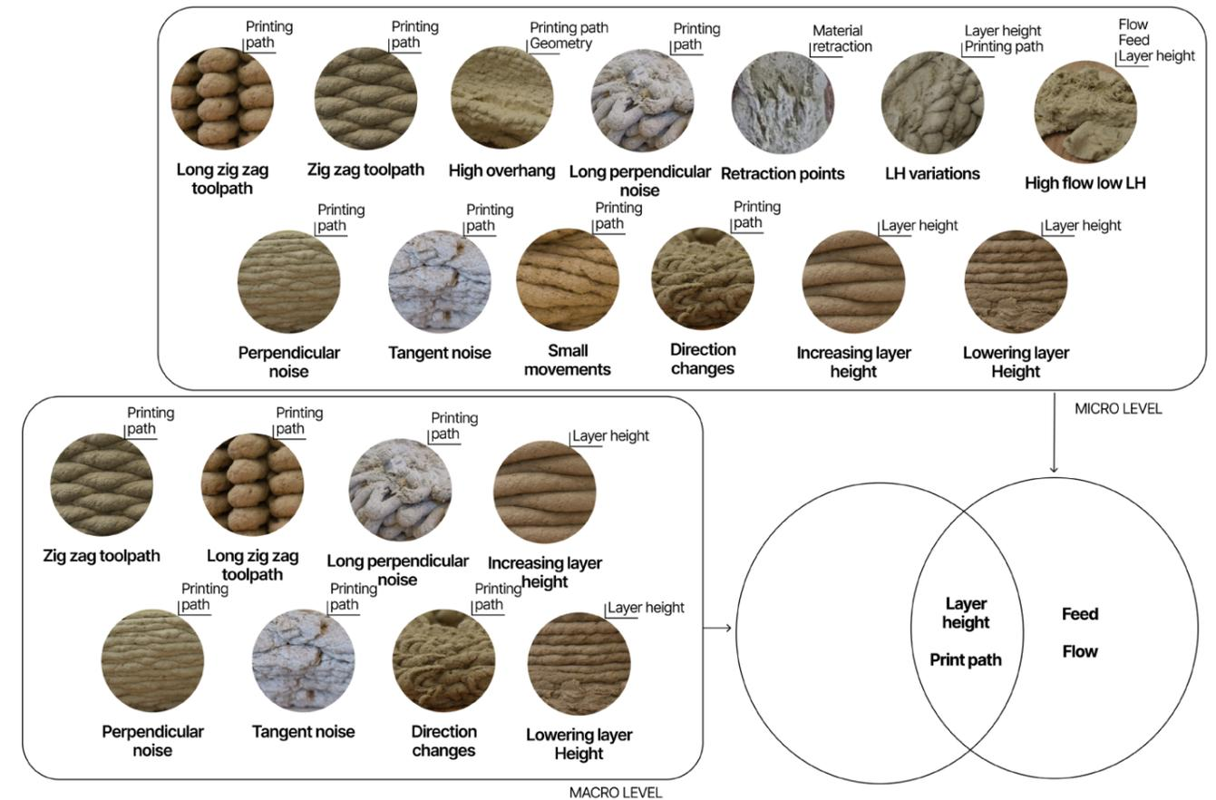
Figure 15: Parameters contributing to the roughness of BM-1 with micro and macro influence
