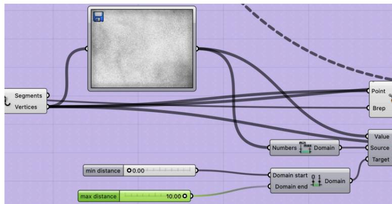
The noise was generated through image mapping. For this example a grainy image was used. The point movement distances were mapped to a maximum of 10mm. To hide the seam, the prototype's polyline was spiralled using 40 points for the precision ramp.
