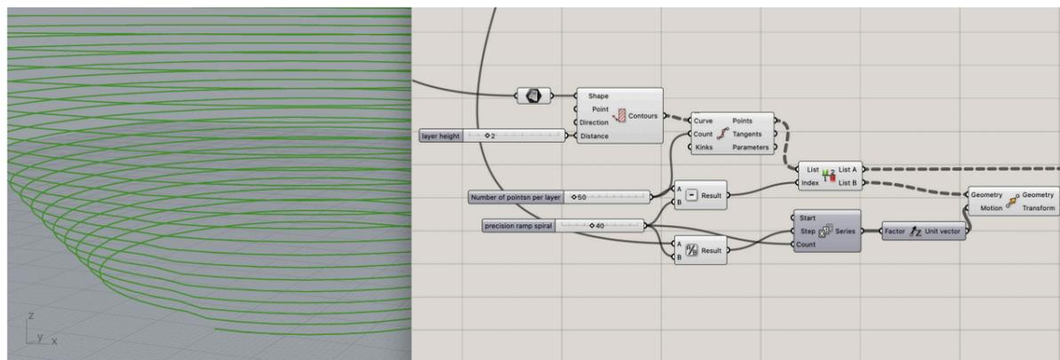
To hide the seam, the prototype's polylines were spiraled using 40 points for the precision ramp.
