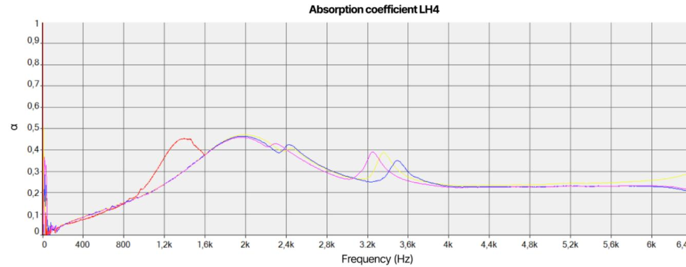
Figure xx: Comparison of absorption coefficients of the same sample (LH4), replacing it in the tube for every measurement
