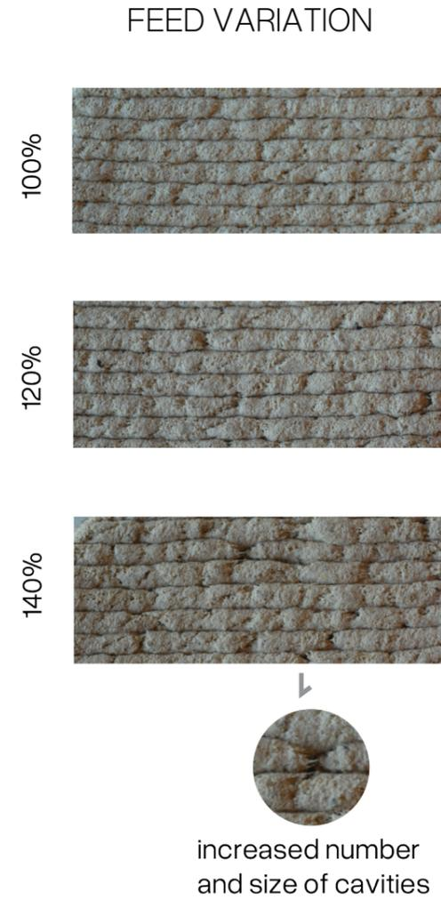
Figure 22 : Cavity formation due to feed increment
