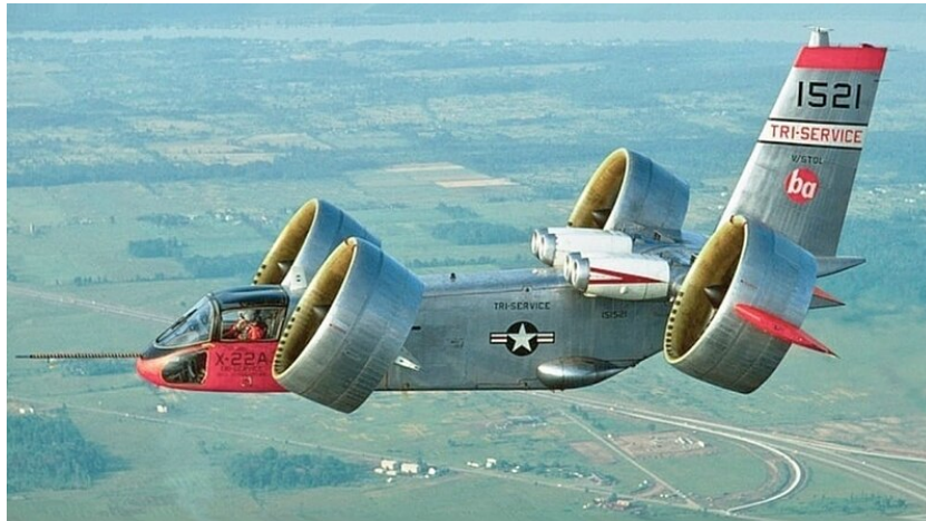
Figure 2.4: Bell X-22 (US Army, 1965) VTOL aircraft. This VTOL test bed is an application of ducted propellers.
