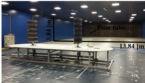
Figure 3.6: Two-sail arrangement mounted on the wind-tunnel turntable
