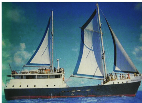
Figure 1.2: The Fijian ferry Na Mata-i-sau retrofitted with soft sails. (Photo: Nuttall et al., 2014 )
