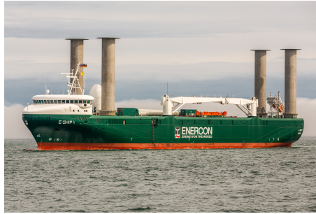
Figure 5.1: The E-ship 1 is a wind-assisted ship equipped with four Flettner rotors. Photo: Alan Jamieson
