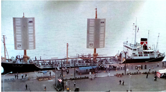
Figure 1.3: Shin Aitoku Maru , the first ship to be fitted with the JAMDA-NKK wing sails. (Photo: MK)
