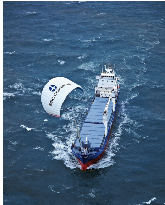
Figure 2.2: A ship sailing with the assistance of a kite sail. (Photo: Skysails)
