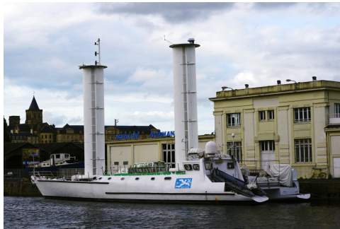
Figure 2.1: Alcyone , the Research Expedition Vessel of the French Cousteau Foundation equipped with two Turbosails. (Photo: David Merrett)
