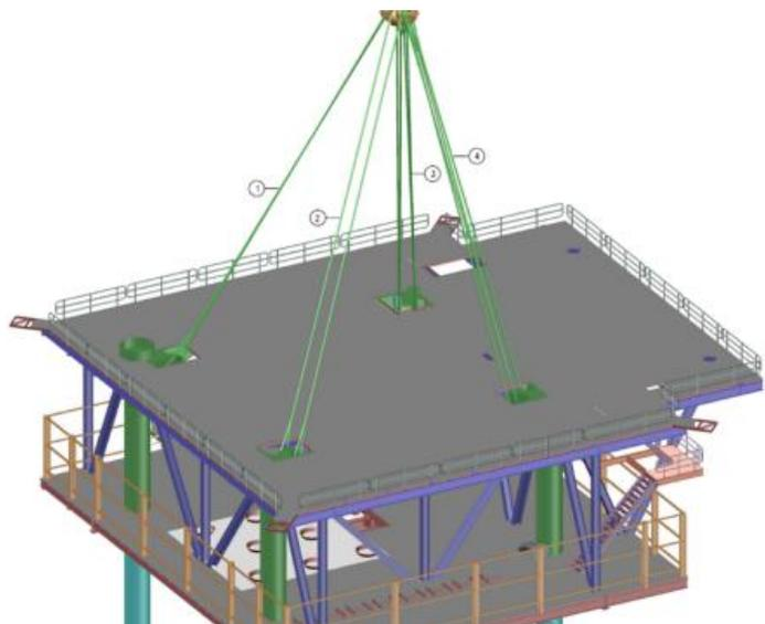
(b) Rigging and lift point configuration of JD topside
