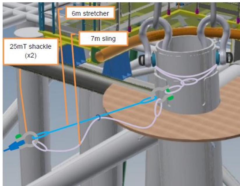
Figure 3.18: L10 jacket lift point and tugger connection
