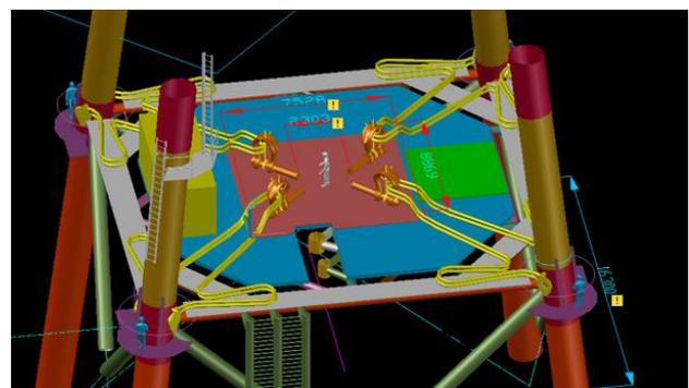
(b) Rigging and lift point configuration of UR jacket
