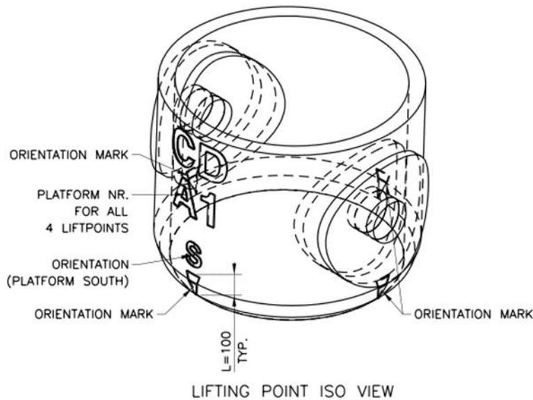
Figure 3.5: Prefabricated piece of leg with two reinforced holes.
