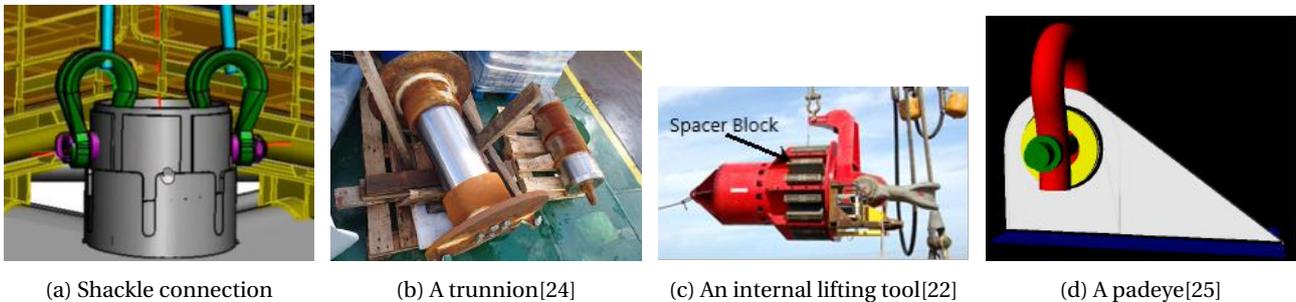
Figure 1.6: Four common lift points
