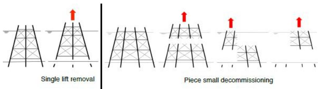
Figure 2.2: Difference single lift and piece-small [27]
