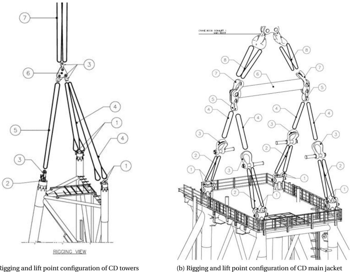
Figure 3.7: CD jacket lift point configuration
