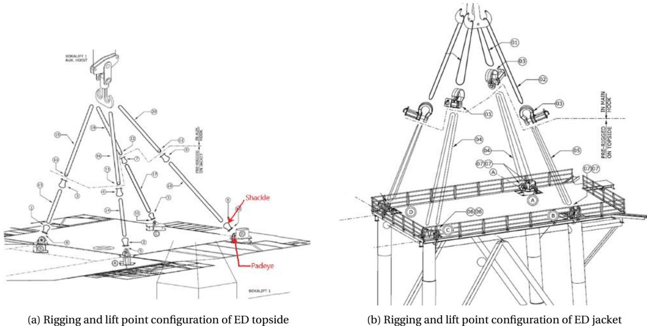
Figure 3.8: ED platform lift point configuration
