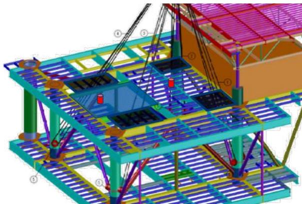
(a) Rigging and lift point configuration of UR topside
