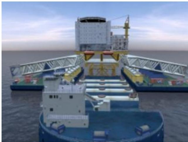
Figure 2.3: The Twin Marine lifter single lift system
