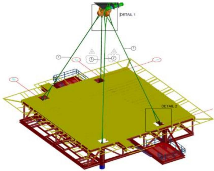
(b) Rigging and lift point configuration of JD helideck
