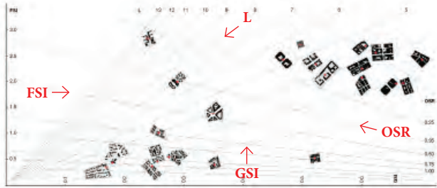
Figure 4/02a: Spacematrix diagram plotting GSI and FSI which helps define the 'physical density' or urban form.
