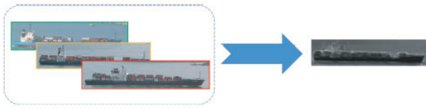
Figure 3-4: MACH filters combine a collection of training images (left) into a single composite template (right) by optimizing a set of metrics, [9].
