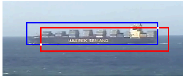
Figure 4-3: Illustration of a ground truth (GT, blue rectangle) and a bounding box produced by a detection algorithm (BB, red rectangle).
