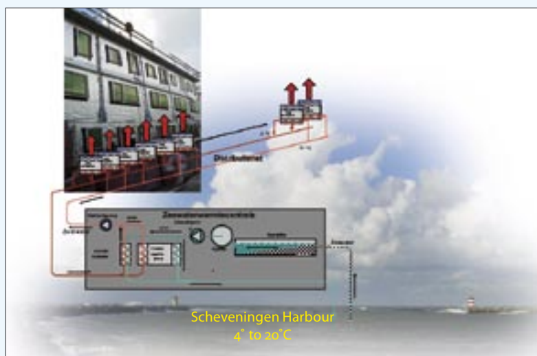
Commissioned by the Vestia/Ceres housing corporation, the Deerns company of engineering consultants have developed a plan to heat 750 new houses in the Duindorp quarter of Scheveningen within the next three years using a seawater heat plant located in the harbour. The houses will feature individual heat pumps connected to the plant’s source heat network.
