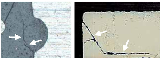
Figure 3: Fractures within package body (left) and silicon (right).
