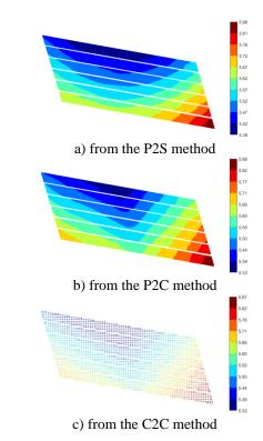
Figure 6. Vertical clearance values from the proposed methods when the road surface is used as a reference surface (Unit in meter)
