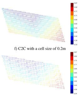
g) C2C with a cell size of 0.4m Figure 5. Vertical clearance values of the bridge as obtained by the proposed methods (Unit in meter)
