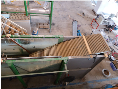
Figure 3.3: Wave Absorber at the end of the flume
