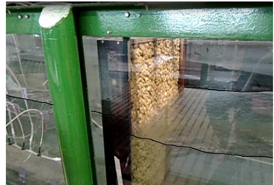
Figure 4.2: Trough of the wave in front of the block, note the water level difference over the block.
