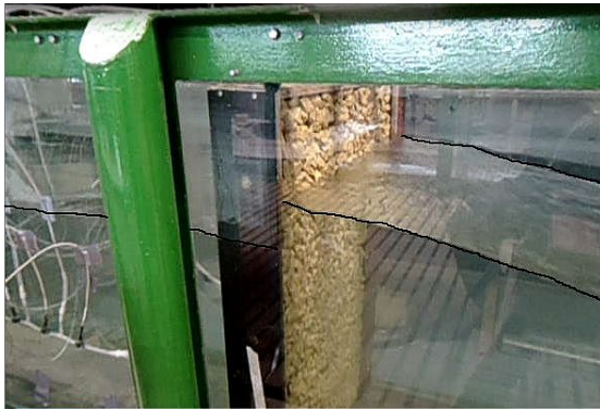
Figure 4.1: Peak of the wave in front of the block, note the water level difference over the block.
