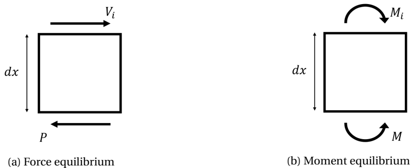
Figure 4.4: Equilibrium condition at x = L_1 for an element with size dx
