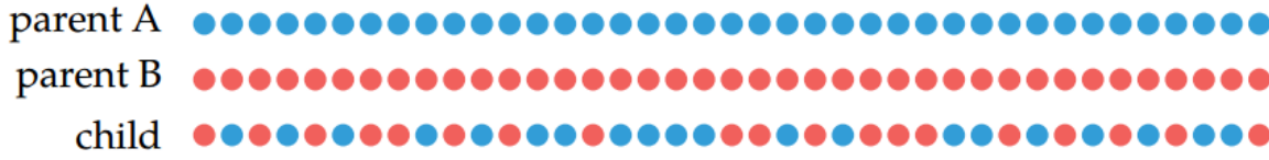
Figure 2.4: A representation of the genes of a child, as inherited by the parents via a uniform-crossover operation [51].
