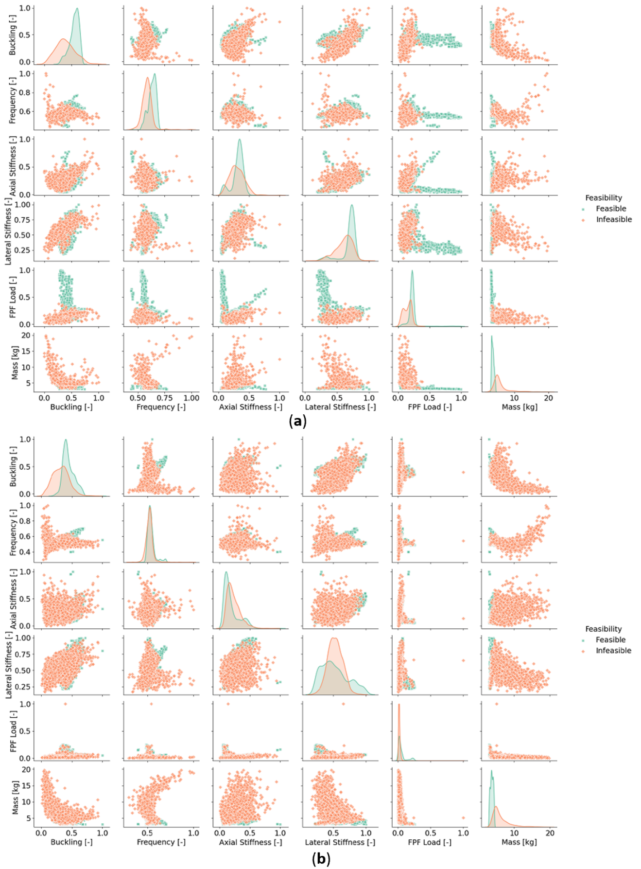
Figure 4.31: Design feasibility with respect to the imposed constraints for the CV case with a) 3 and b) 4 CPs.
