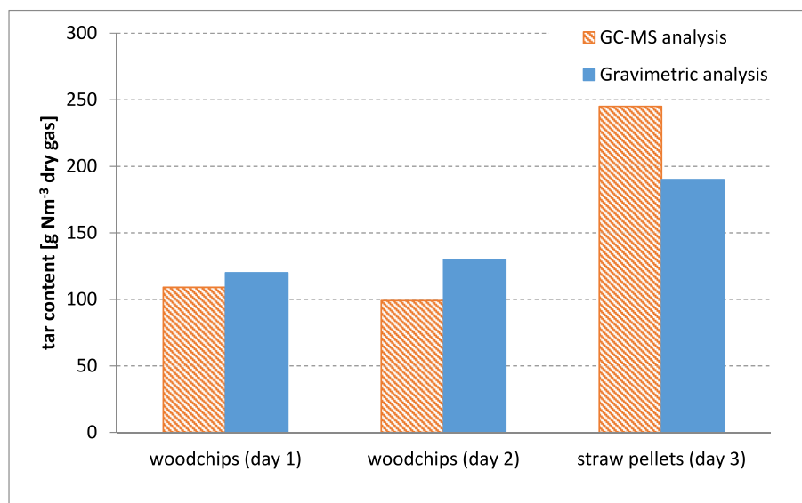
Fig. 4. Comparison of gravimetric (dashed) and GC-MS (solid) analysis.
