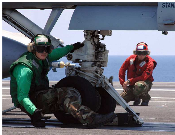
Figure 3-6: Attachment of the F-14 with the shuttle of the steam catapult [42]
