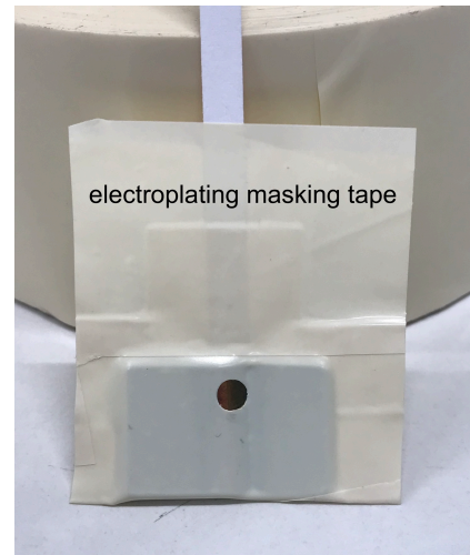
(b) Sample masking (3M™ electroplating tape 470)
