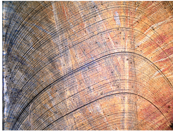
Figure 4.6: OMx100 - Lap joint weld before H 2 exposure, no etched
