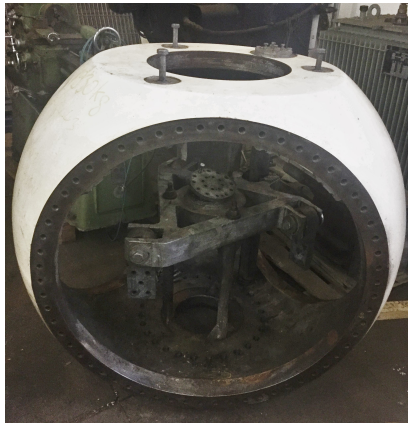
Figure 2-25: Original Vestas V44 hub, with in the middle the triangular pitch traverse.
