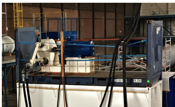
Figure 2-23: Mechanically coupled Pelton turbine and generator. The two variable spear valves are pointed towards the Pelton turbine buckets (located in the white housing).
