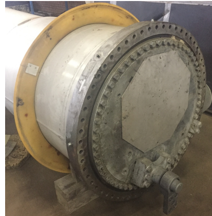
Figure 2-26: Blade-to-hub bearing, with below the traverse connection link.
