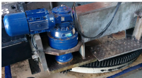
Figure 4-17: One of the two yaw motors driving the small pinion gear against the large bull gear
