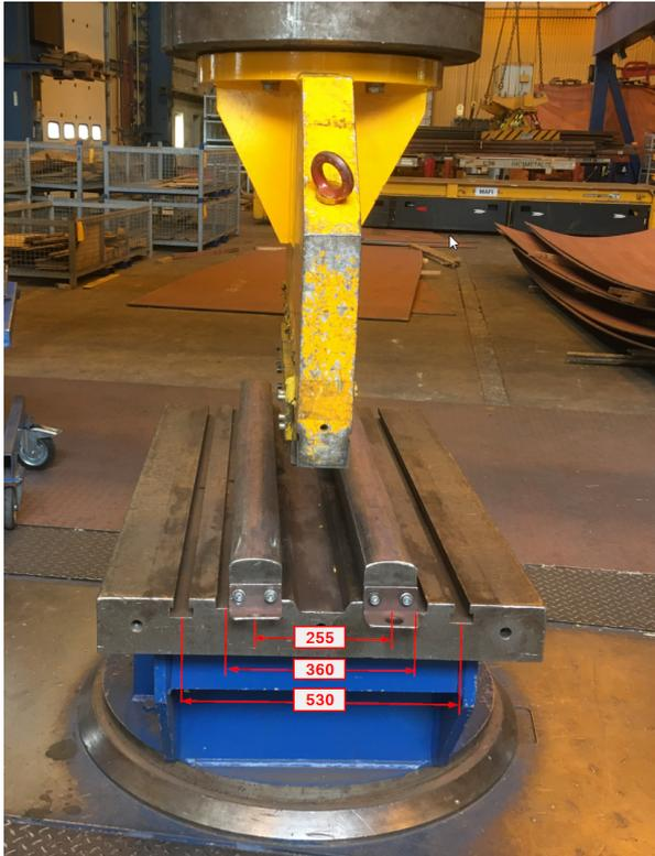
Figure 3.6: Three point bending machine at IHC, dimensions are in millimeter [1]
