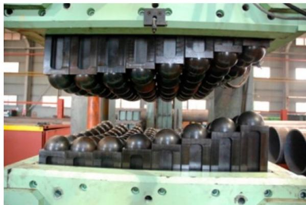
Figure 2.2: Multi point forming machine used in research by Hwang and Lee [10]
