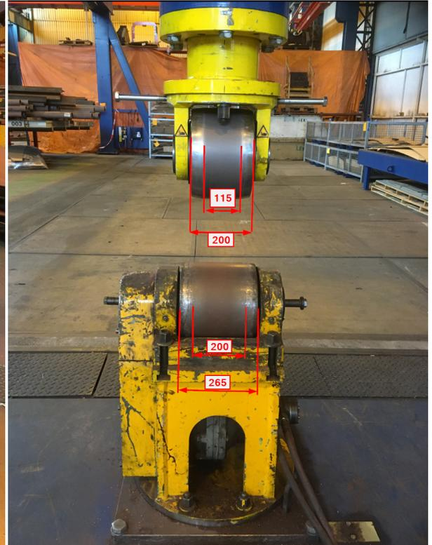
Figure 3.7: Rolling machine at IHC, dimensions are in millimeter [1]
