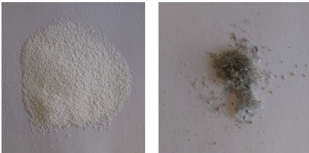
Figure 3.13: Cellulose acetate before (left) and after (right) washing
