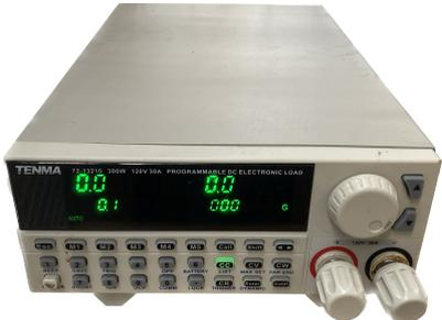
Figure B.3: 72-13210 DC Electronic Load from Tenma
