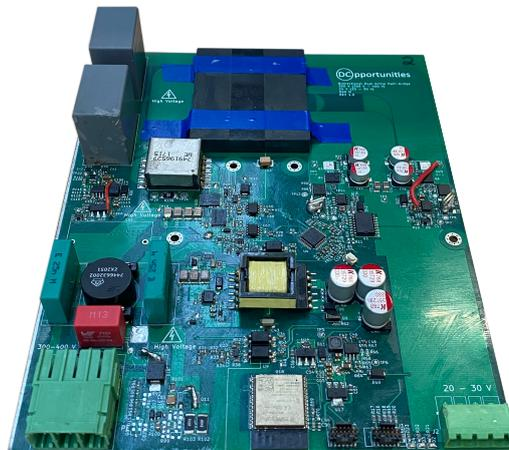
Figure B.1: DAHB converter prototype
