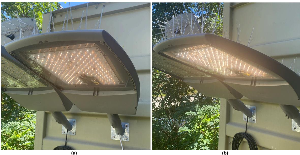
**Figure 6.21:** LED droop control testing (a) DC microgrid voltage is 321V: droop mode (b) DC microgrid voltage is 380V: constant power mode
