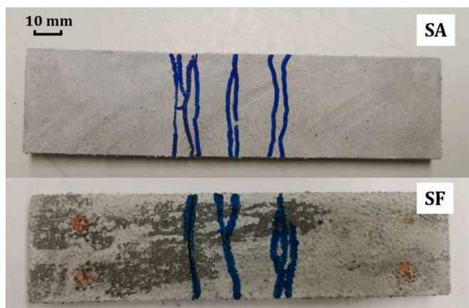
Fig. 13. Specimen with multiple cracks after four-point-bending test.
