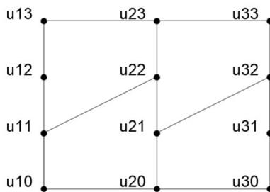
**Figure 68.** Displacement nodes in a double braced system.
