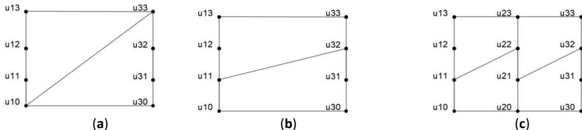
**Figure 65** Schematization of three braced frames: (a) Concentrically single braced, (b) Eccentrically single braced, (c) Eccentrically double braced frame (own work).
