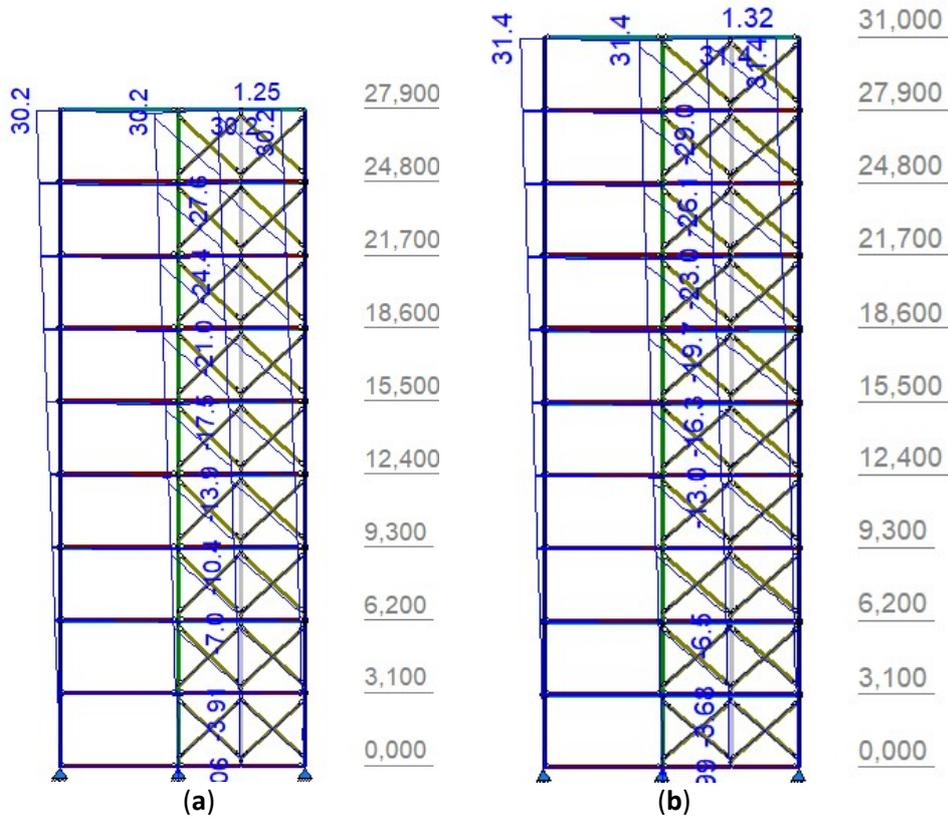
Figure 123. Horizontal displacements Variant 2 O-F: (a) 9 storey model, (b) 10 storey model.
