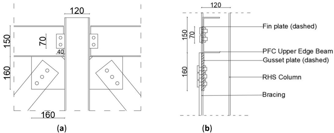
**Figure 51.** Bracing connection below ceiling height: (a) Side view, (b) Cross-section (own work).
