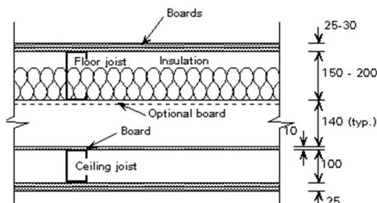
Figure 4. Standard floor and ceiling system (Steelconstruction.info).
