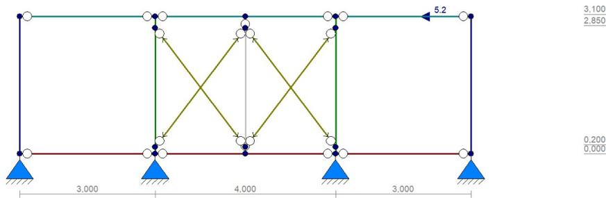
Figure 44. Single module structural model in (Technosoft).
