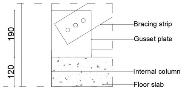
**Figure 52.** Side view of lower bracing connection.
