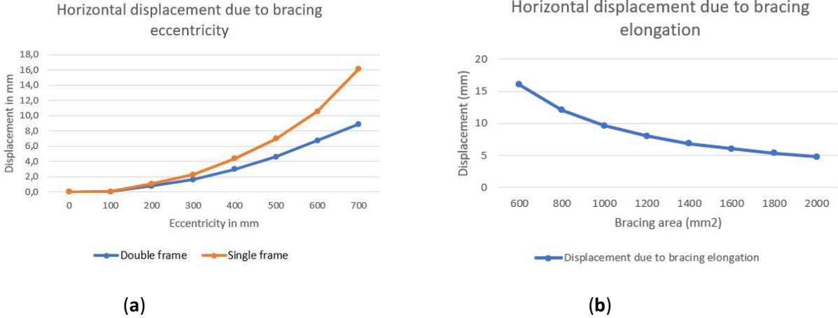
**Figure 74.** Horizontal displacement due to bracing geometry: (a) Support eccentricities, (b) Profile area.
