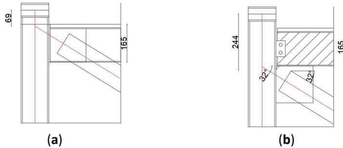
**Figure 60.** Upper bracing eccentricities using PFC-section support: (a) Single frame, (b) Double frame (own work).
