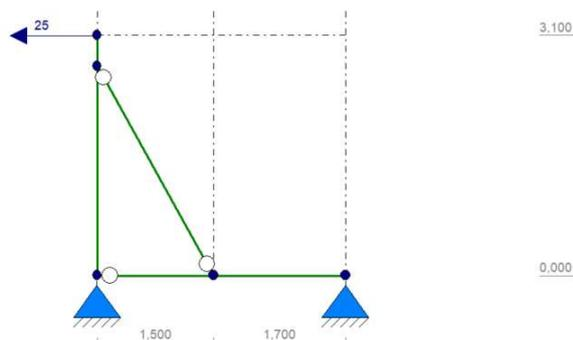
**Figure 69.** Geometry and applied load on a braced column (Technosoft).
