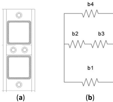
**Figure 106** Gunawardena inter-module connection: (a) Top view, (b) Schematization of longitudinal bolt stiffness.
