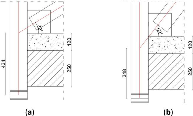
**Figure 59.** Lower bracing eccentricities using PFC-section support: (a) Single frame, (b) Double frame (own work).
