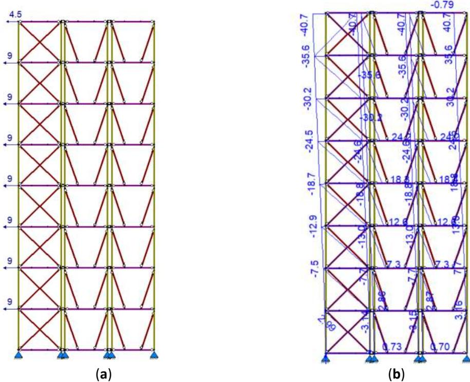
Figure 116. Variant 2.2 Strips: (a) Geometry and wind load, (b) Horizontal displacement for governing load combination.
