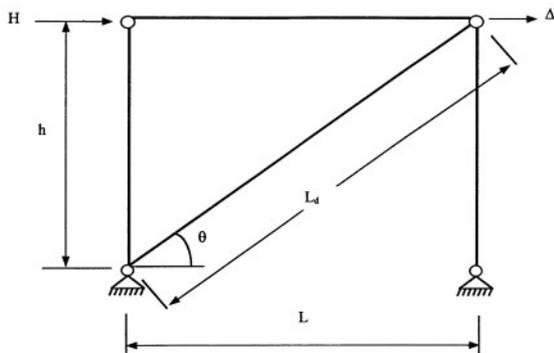
**Figure 66.** Parameters in a braced structure.
