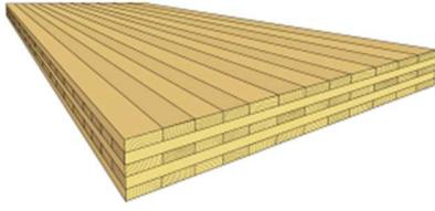
**Figure 11.** Lamination of lamellae into a CLT panel.
