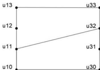
**Figure 67.** Eccentrically braced frame.
