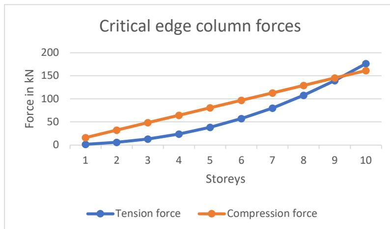
**Figure 73.** Calculation of critical column forces in transverse direction.
