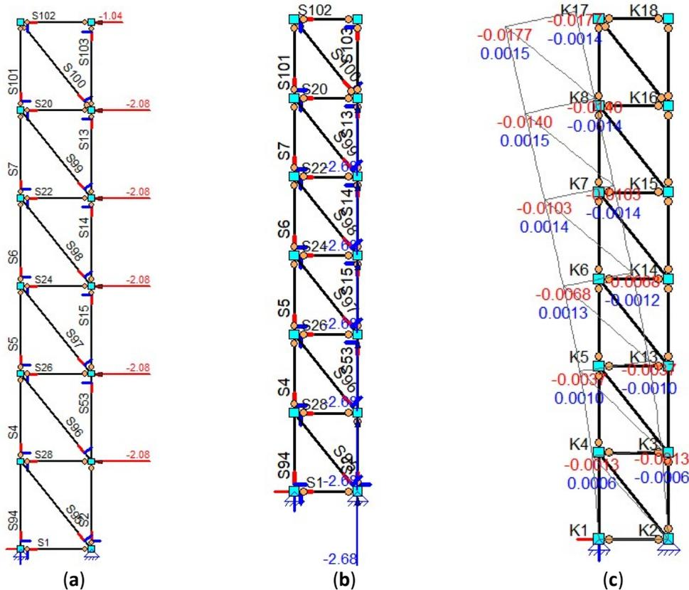
**Figure 28.** Matrixframe horizontal verification: (a) Wind load (kN), (b) Shifted permanent load, (c) Horizontal displacements.
