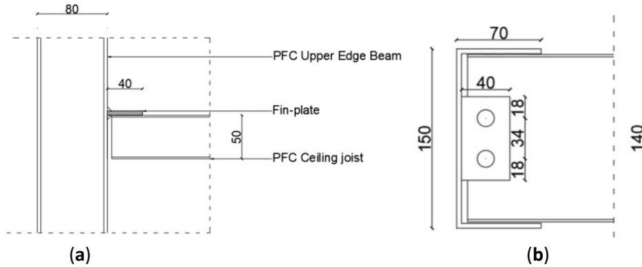
**Figure 62** Ceiling joist-Edge beam connection: (a) Top view, (b) Cross-section (own work).
