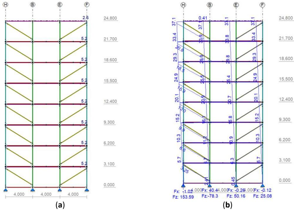
Figure 110. Variant 1 S-O-S: (a) Geometry and wind load, (b) Horizontal displacement on governing load combination.
