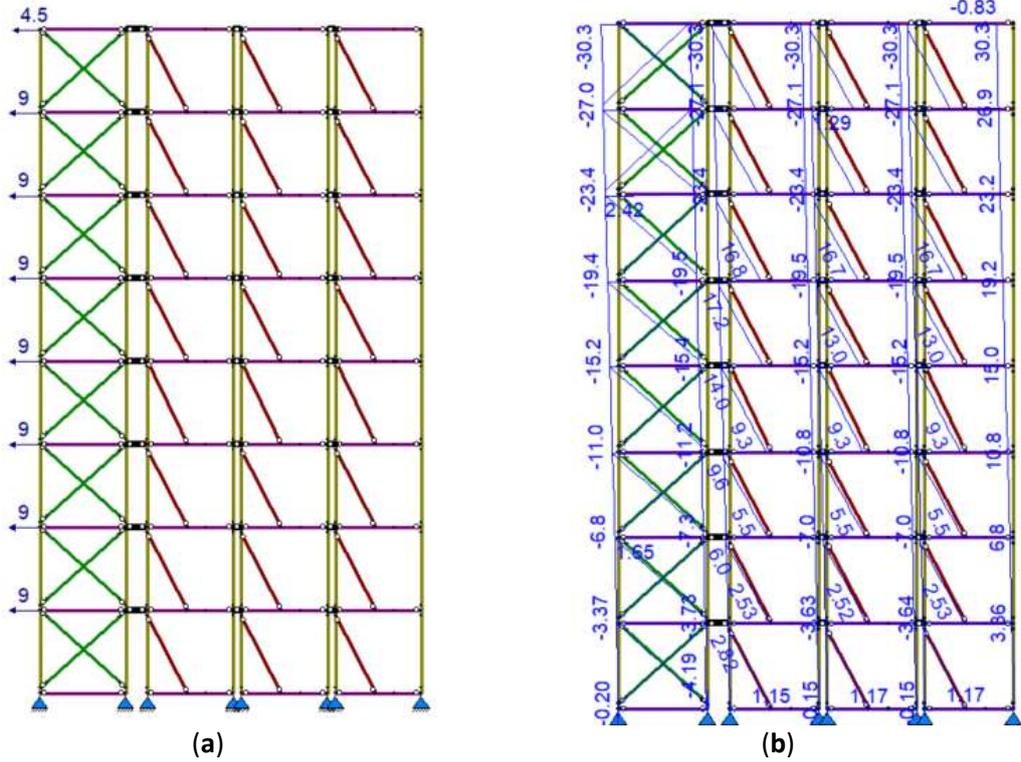
Figure 118. Variant 3.2 Mix: (a) Geometry and wind load, (b) Horizontal displacement for governing load combination.
