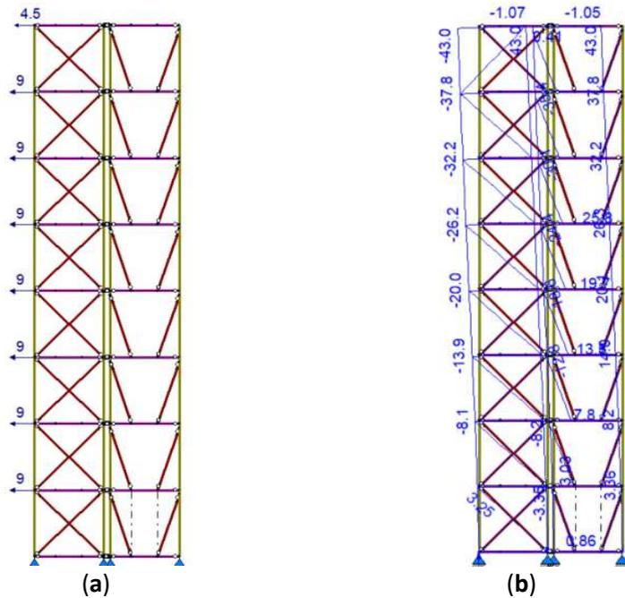
**Figure 115.** Variant 2.1 Strips: (a) Geometry and wind load, (b) Horizontal displacement for governing load combination.
