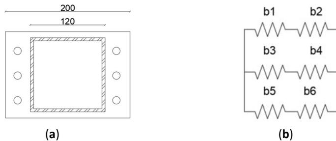
**Figure 107** Styles inter-module connection: (a) Top view, (b) Schematization of longitudinal bolt stiffness.
