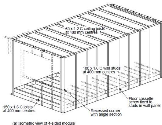
**Figure 25.** Isometric view of a 4-sided module (Lawson et al., 2010).
