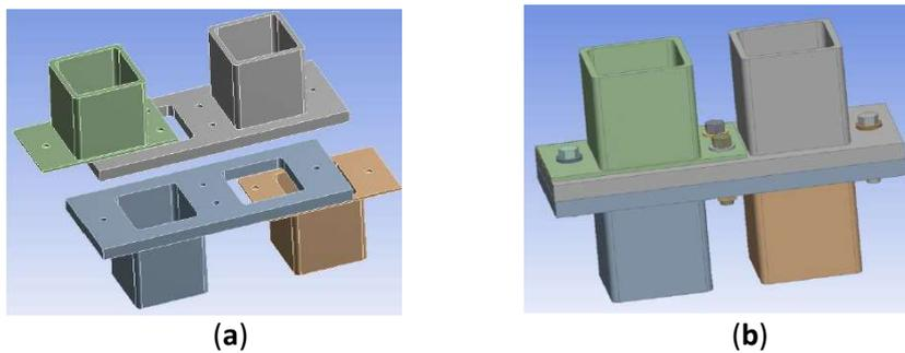
**Figure 54.** Gunawardena Joint 3D schematizations: (a) Order of module installation, (b) Post installation and bolting (Gunawardena et al, 2016).
