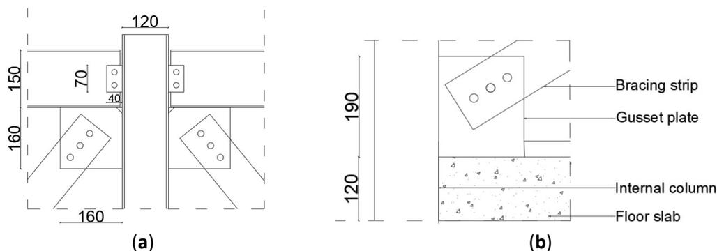
**Figure 63.** Bracing to gusset plate connection: (a) Upper connection, (b) Lower connection (own work).
