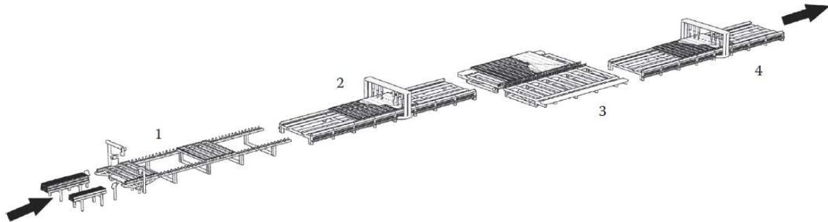
**Figure 14.** Semi-automated line for wall and ceiling panels (Lawson et al., 2010).
