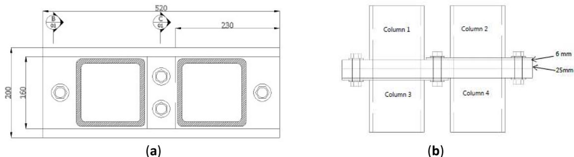
**Figure 55.** Scheme of bolt interaction: (a) Top view, (b) Side view (Gunawardena et al).
