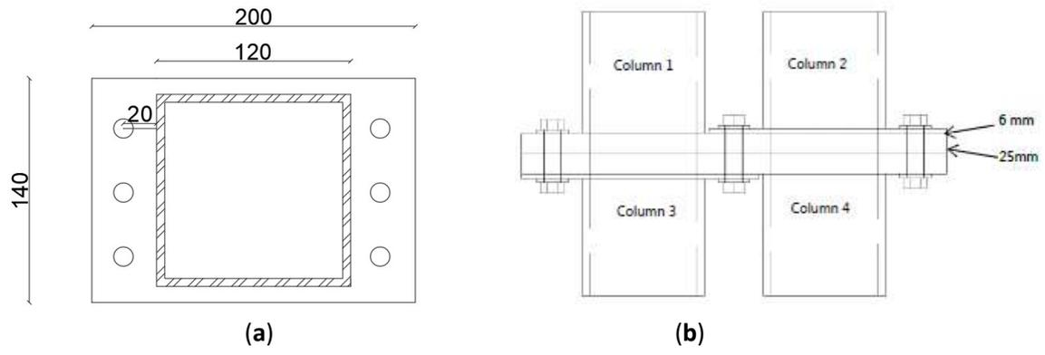
**Figure 108.** Inter-module joint schemes: (a) Top view, (b) Cross-section.
