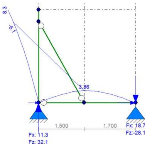
Figure 70. Deformed state of a braced column (Technosoft).
