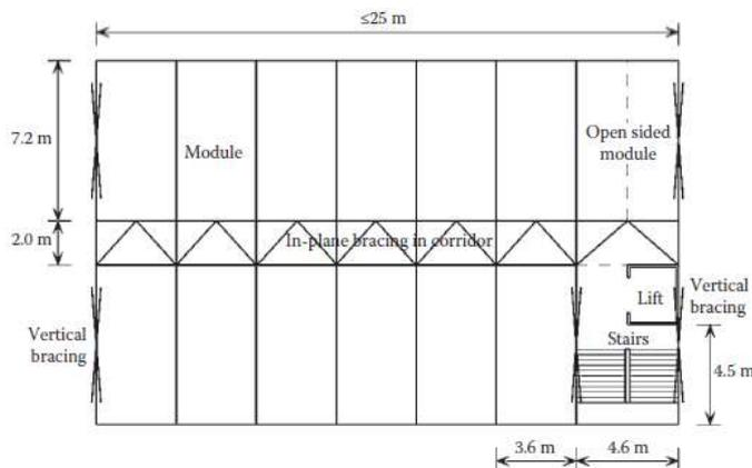
**Figure 16.** Location of vertical and horizontal bracing (Lawson et al., 2010).
