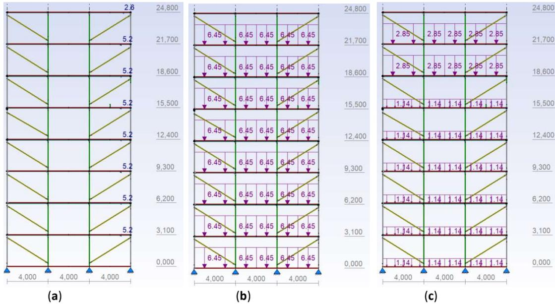
**Figure 109.** Variant model loads: (a) Wind load, (b) Permanent load, (c) Variable load.
