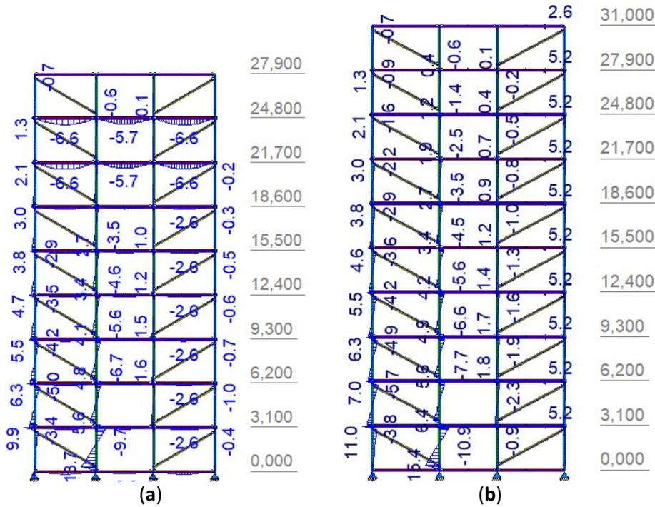
Figure 120. Internal moments Variant 1 S-O-S: (a) 9 storey model, (b) 10 storey model.
