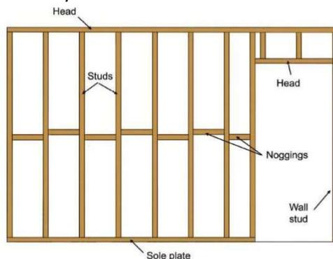
**Figure 10.** Timber stud wall.
