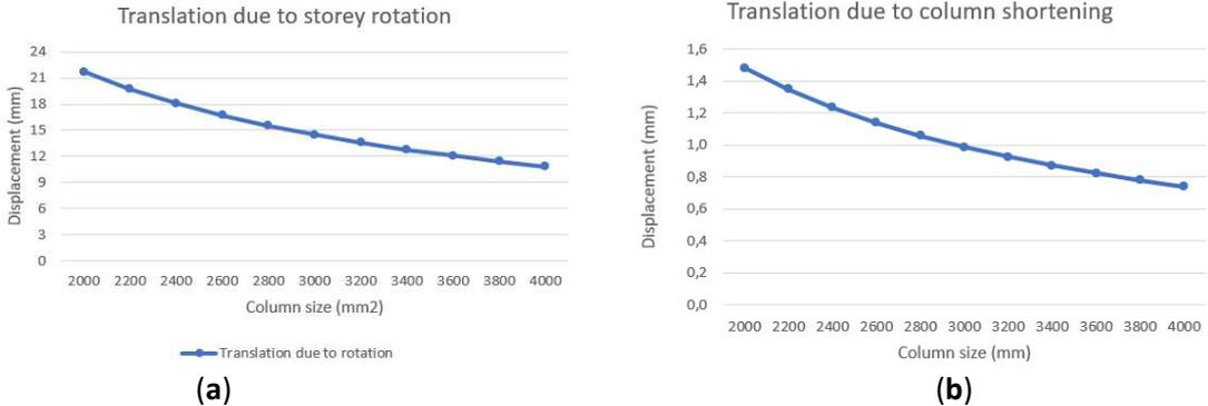
**Figure 75.** Displacements for different column sizes: (a) Due to storey rotation, (b) Due to column shortening.
