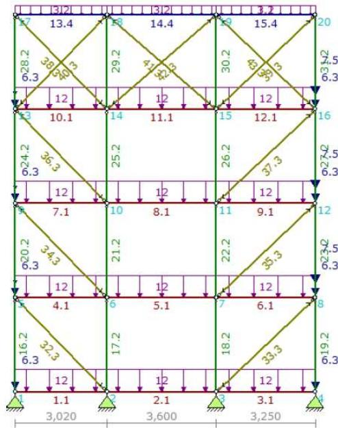
**Figure 37.** Longitudinal stability scheme (Pieters Bouwtechniek).
