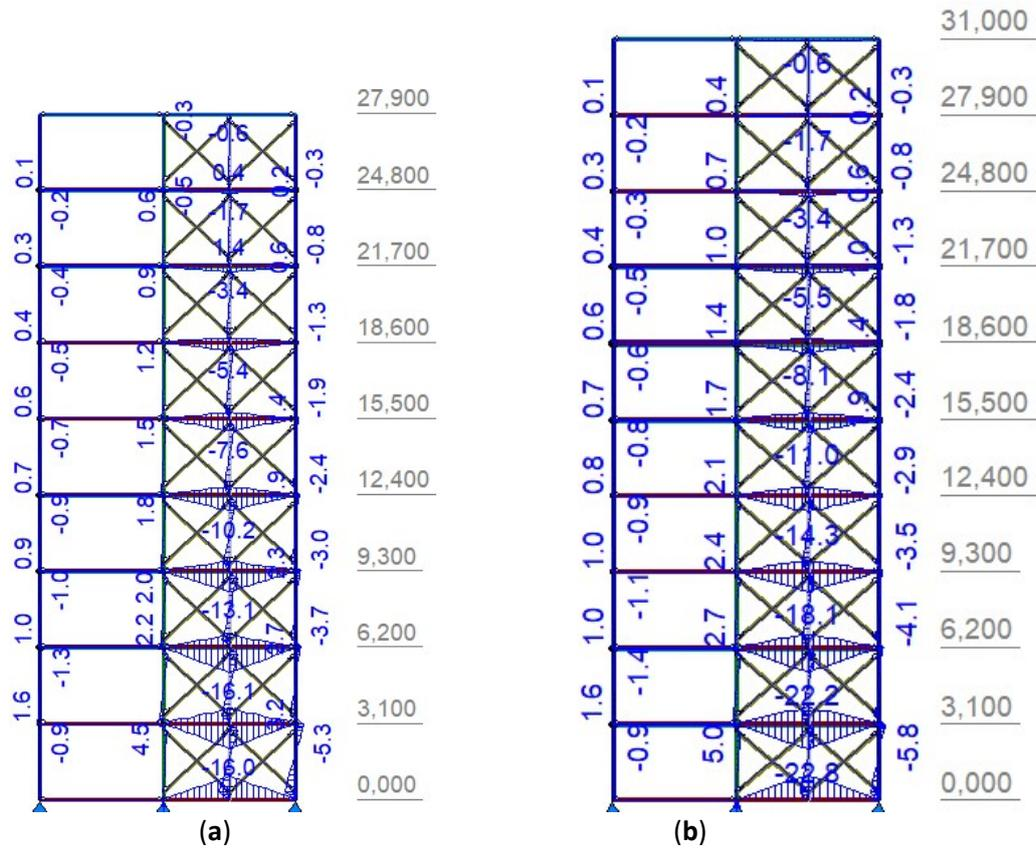
Figure 122. Internal moments Variant 2 O-F: (a) 9 storey model, (b) 10 storey model.
