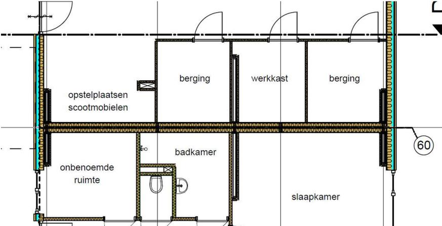
Figure 39. Location of bracings in floor plan (Pieters Bouwtechniek).
