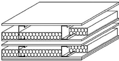
Figure 3. Light steel joists for ceiling with next floor on top (Lawson et al).
