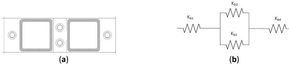
**Figure 105.** Gunawardena inter-module connection: (a) Top view, (b) Schematization of transverse bolt stiffness.
