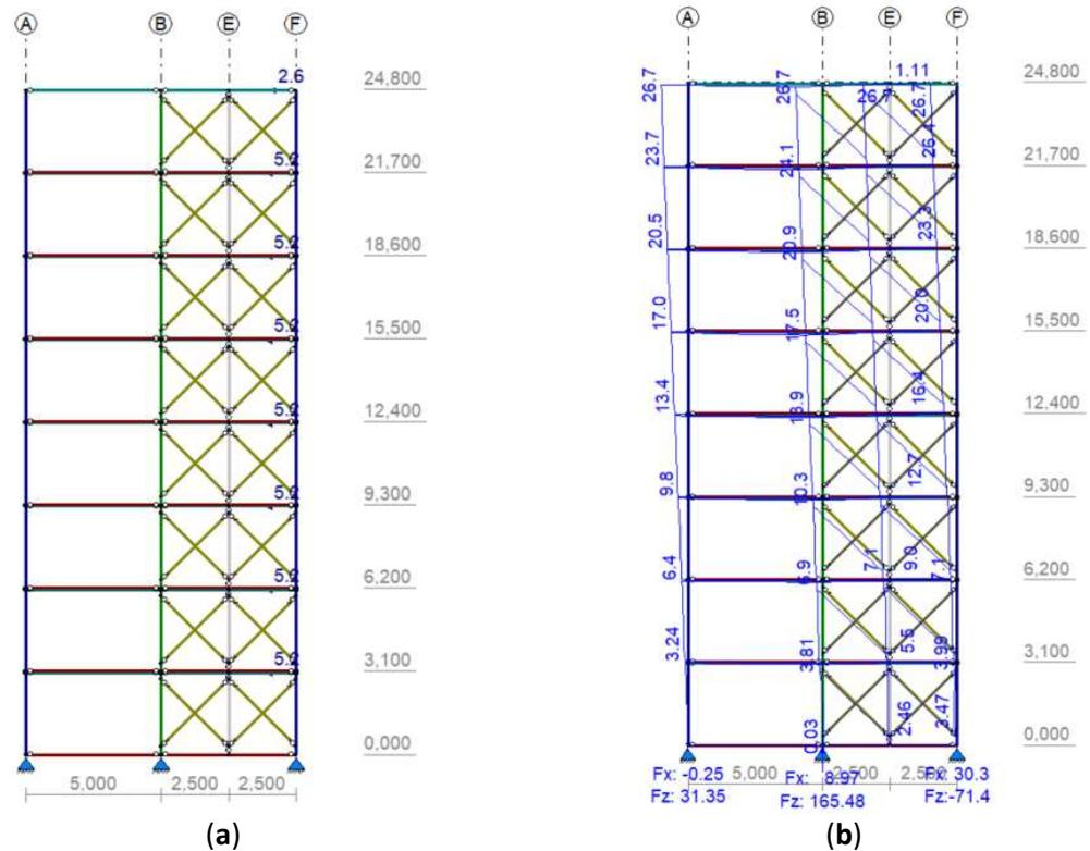
Figure 111. Variant 2 O-F: (a) Geometry and wind load, (b) Horizontal displacement on governing load combination.
