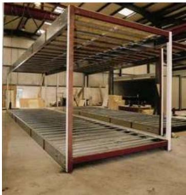
**Figure 13.** Open-sided module (Kingspan).
