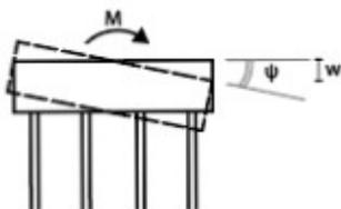
**Figure 61.** Base rotation of the foundation during wind.
