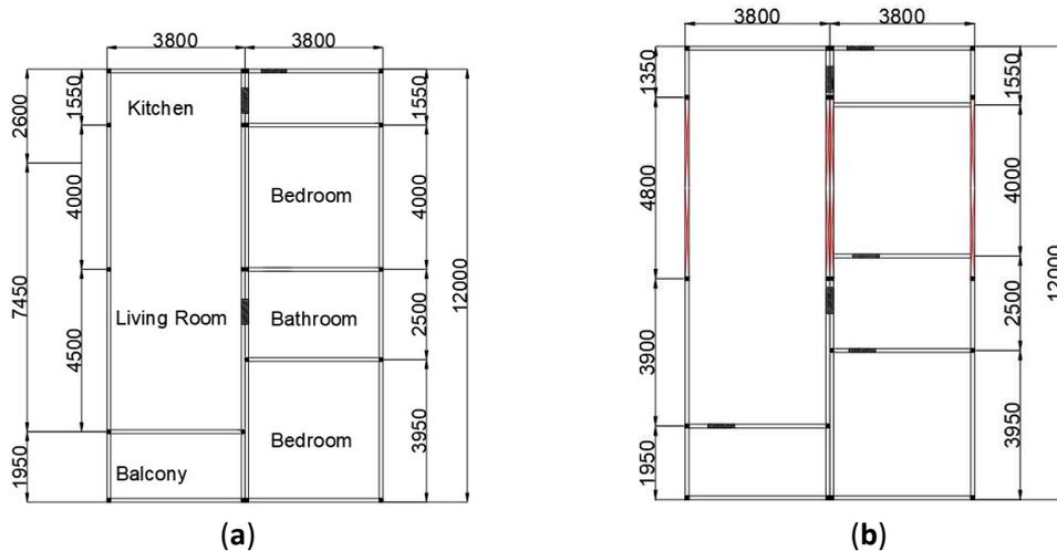
**Figure 26.** Raines Court floor plans: (a) Functional, (b) Structural (own work).
