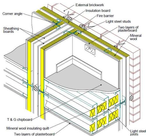
**Figure 8.** Fire safety measures in wall and floor structure (Lawson, 2007).
