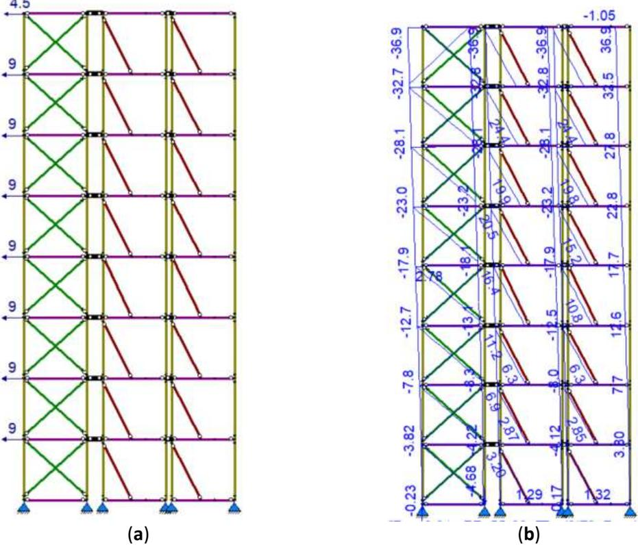
Figure 117. Variant 3.1 Mix: (a) Geometry and wind load, (b) Horizontal displacement for governing load combination.
