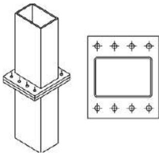
**Figure 56.** Bolted plates inter-module connection (Styles et al).
