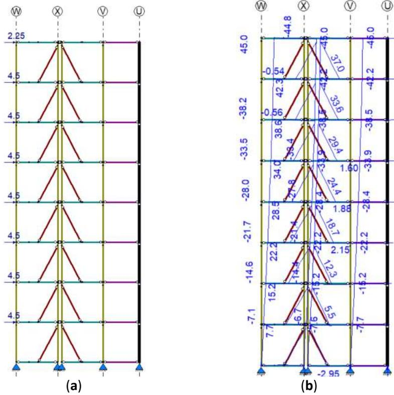
**Figure 114.** Variant 1.1 Box profiles: (a) Geometry and wind load, (b) Horizontal displacement for governing load combination.
