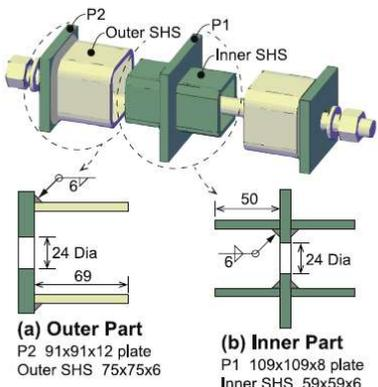
**Figure 58.** Components of shear key inter-module joint (Lacey et al., 2019).
