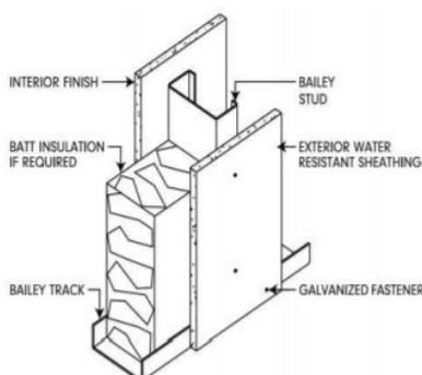
**Figure 41.** Layers in a steel infill wall (Bailey Metal Products, 2019).
