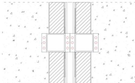
**Figure 57.** Top view of internal column joint (own work).
