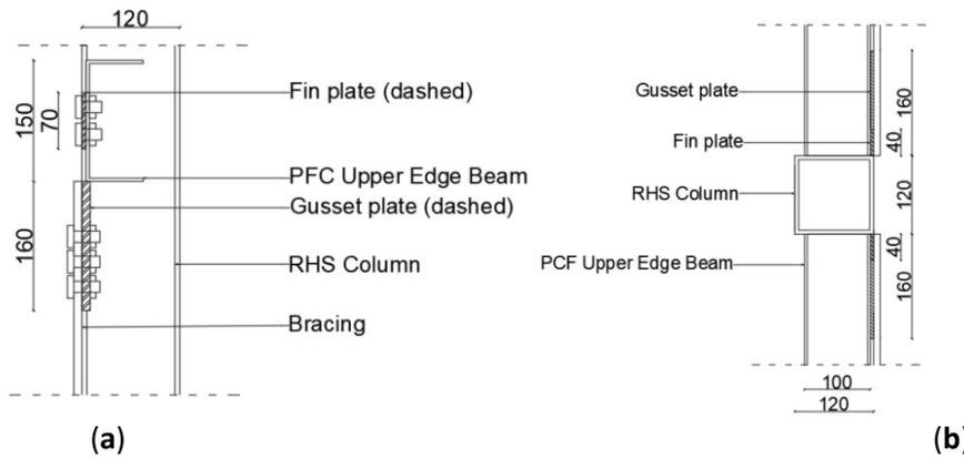
**Figure 64** Connections of fin plate and bracing to column: (a) Cross-section, (b) Top view (own work).
