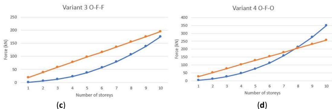
**Figure 72.** Relation between critical tension load and compression load for design variants: (a) S-O-S, (b) O-F, (c) O-F-F, (d) O-F-O (own work).
