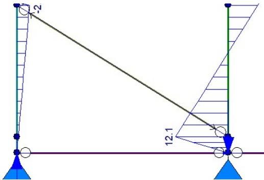
**Figure 119.** Variant 1 S-O-S Governing internal bending moment in 8 storey model (Technosoft).
