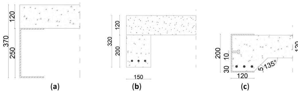
**Figure 50.** Floor slab supports: (a) PFC-section, (b) Concrete beam, (c) Integrated steel-concrete beam (own work).
