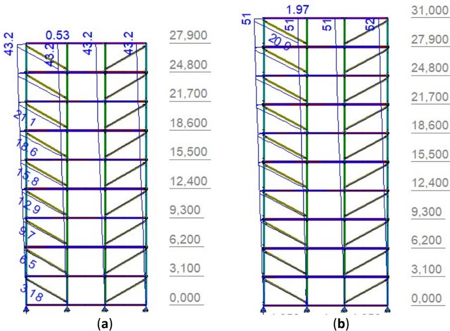
Figure 121. Horizontal displacement Variant 1 S-O-S: (a) 9 storey model, (b) 10 storey model.
