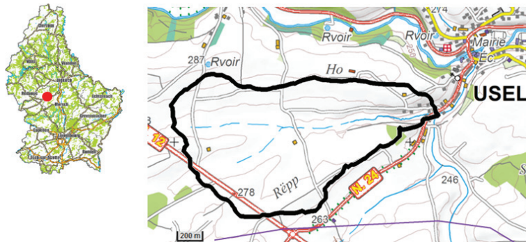
Fig. 6. Catchment area of the Wollefsbach catchment in Luxembourg. Left: red dot indicates the location in Luxembourg, right: topographic map of the Wollefsbach catchment with indicated the catchment boundary of the Wollefsbach catchment (available at: http://eau.geoportail.lu/ ).
