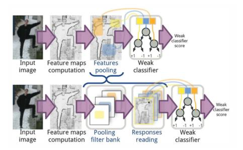
Figure 2.3: Filtered feature channels illustration, for a single weak classifier reading over a single feature channel [2]
