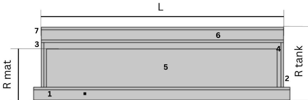
Figure 9: Geometry 4 simulated and compared with the other alternatives. This geometry contains the following domains: 1-coolant fluid, 2-pipe, 3-tank external shell, 4-hydrogen, 5-adsorbent, 6-refrigeration fluid, and 7-external jacket.
