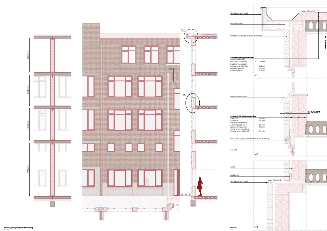
Housing fragment, showing the technologies used for the construction of the building
