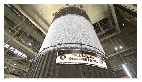
Figure 1.2: Shell Buckling Knockdown Factor test article <sup>2</sup>
