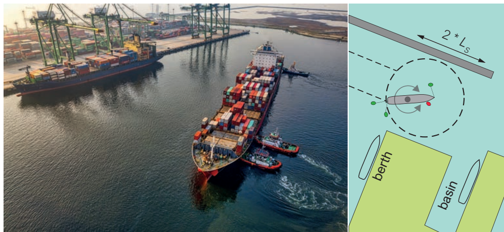
Figure 2.46: Turning a vessel in a turning basin (left: image by william william is free to use under Unsplash Licence; right: image by TU Delft – Ports and Waterways is licenced under CC BY-NC-SA 4.0).
