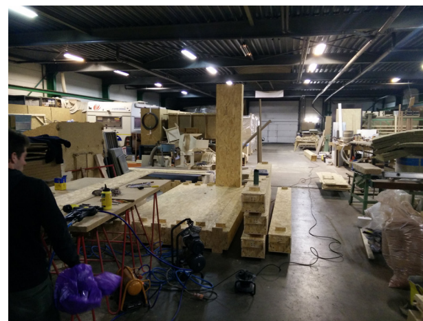
Figure 9.13 a) Milling the final parts and b) Assembling the component off-site (Own illustration)
