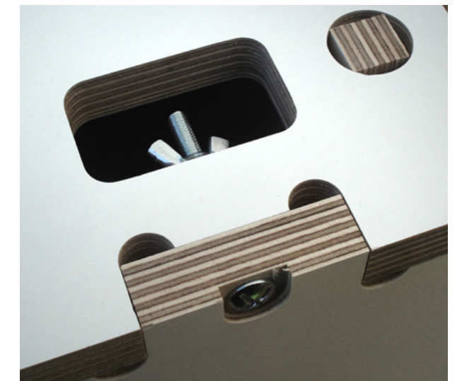
Figure 6.7 CNC-milled bolt/nut connection (raum.fr)
