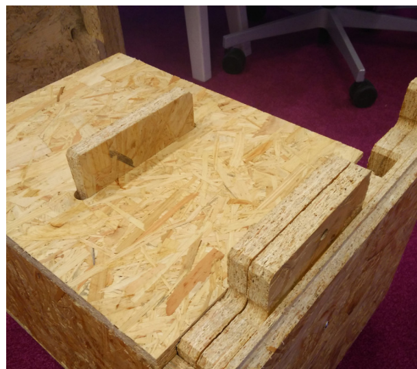
Figure 8.9 Chamfers are required to improve the assembly ease around tight openings (Own illustration)
