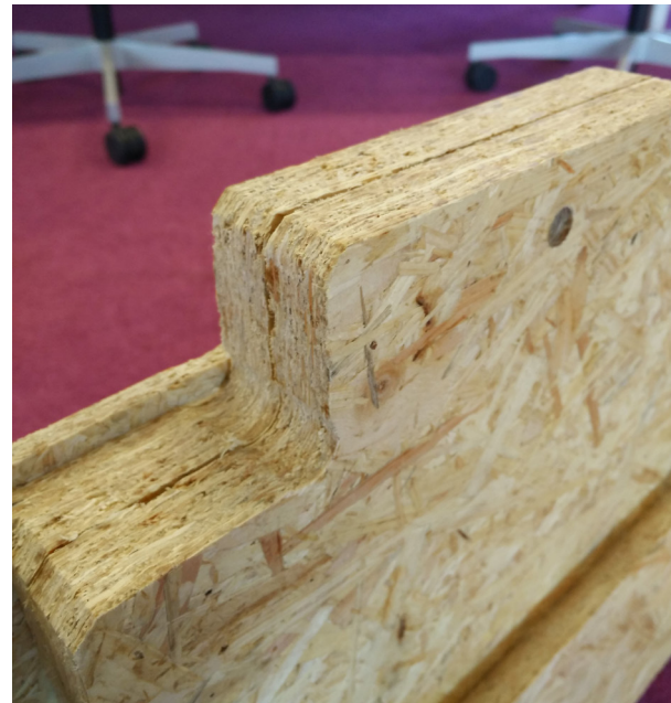
Figure 8.5 Inaccuracies between the different layers of the beam (Own illustration)
