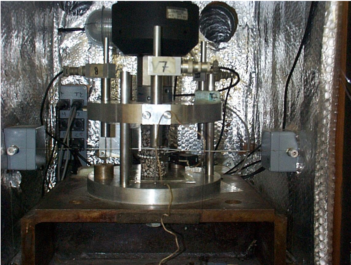
Figure 5.6: Picture from the compression test set-up inside the temperature cabinet
