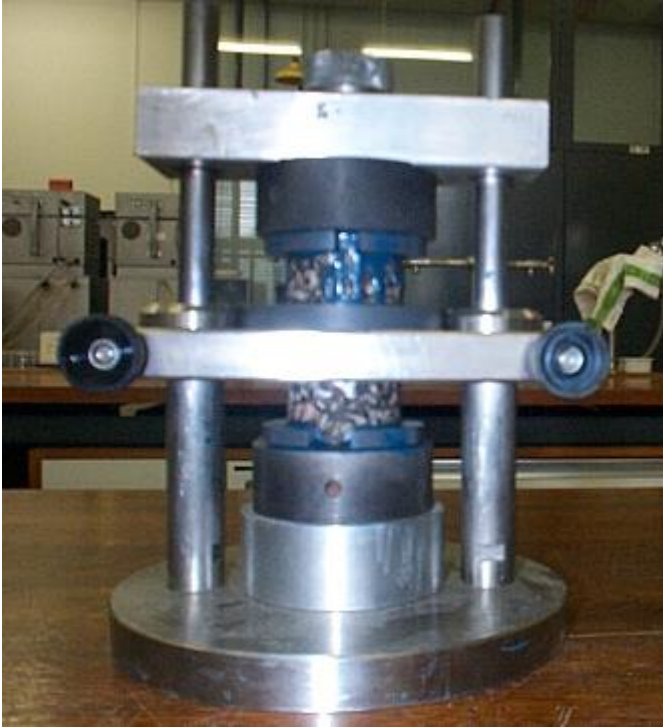
Figure 5.10: Set-up for gluing the caps parallel on the specimen
