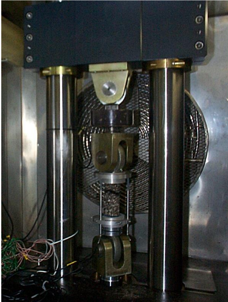
Figure 5.9: Test set up for the uniaxial monotonic tension test
