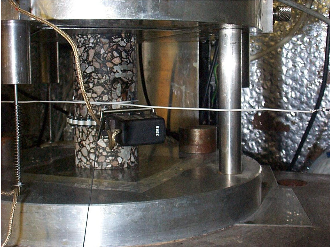
Figure 5.7: Close-up from a specimen inserted in the compression test set-up
